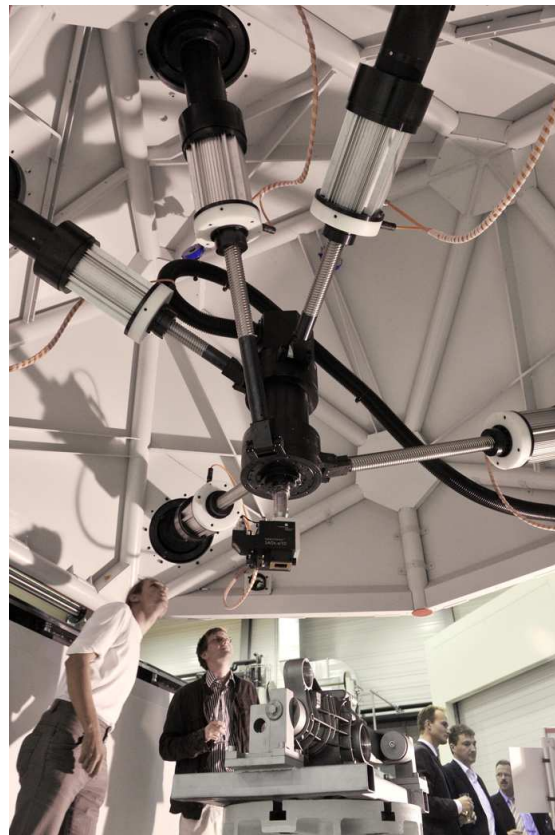
Figure 5.2: A 5-axis milling machine, based on a pentapod, developed by Metrom Mechatronische Maschinen GmbH (reproduced with permission).
