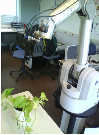
Figure 5. WAM arm used in the experiments holding the Time-of-Flight camera observing a plant.
