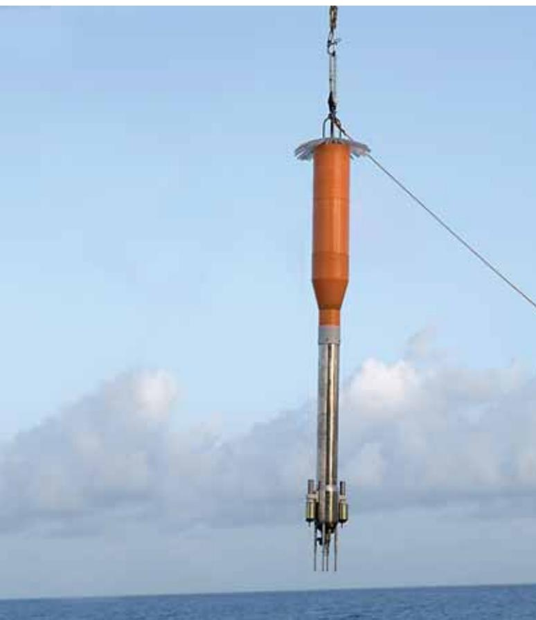
The microprofiler detects the small-scale structure of the ocean, in small eddies (from centimetres to metres) where the mechanical energy is dissipated as heat.
