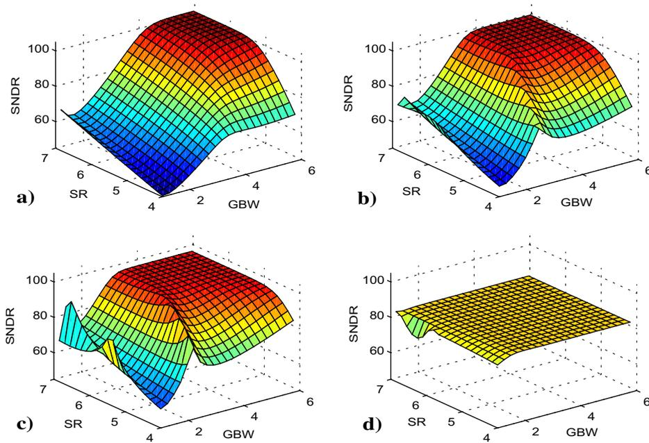
**Figure 5-6: SNRD variation as a function of Slew-Rate and Gain-BandWidth product**
