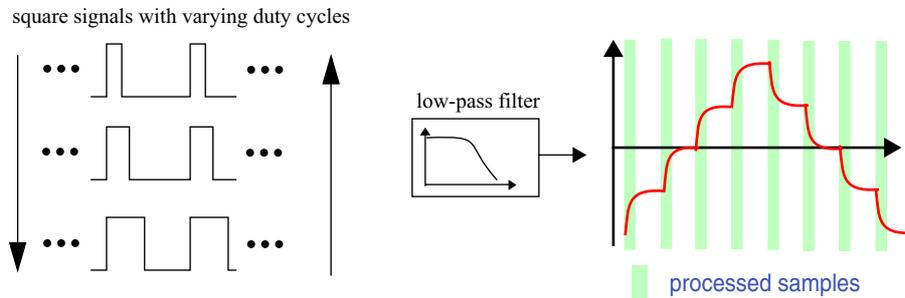
**Figure 2-6: Exponential stepped signal equivalent to a ramp**
