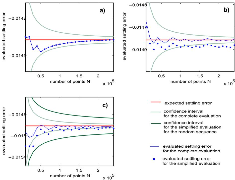
**Figure 5-16:** First order modulator settling error evaluation versus the number of acquired points
