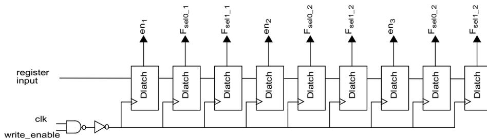
Figure 7-13: Test configuration register
