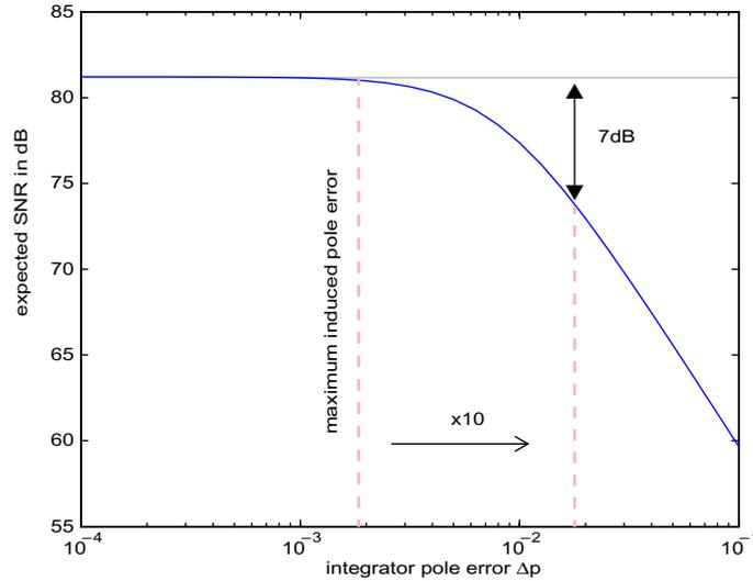
**Figure 7-30:** Expected SNR variation for the prototype as function of the first integrator pole error
