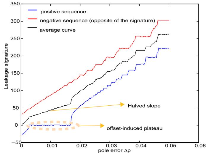
**Figure 4-37:** Signature versus integrator leakage for the alternative leakage test, in the presence of an offset.
