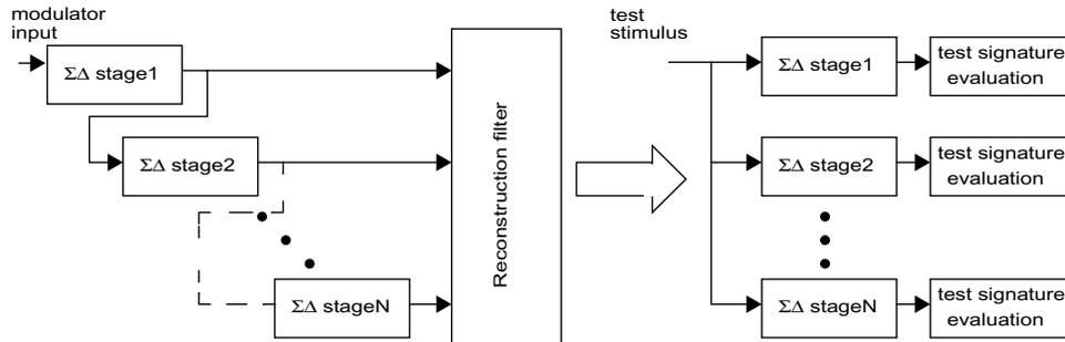
**Figure 3-7: Parallel testing of a cascaded  $\Sigma\Delta$  modulator**
