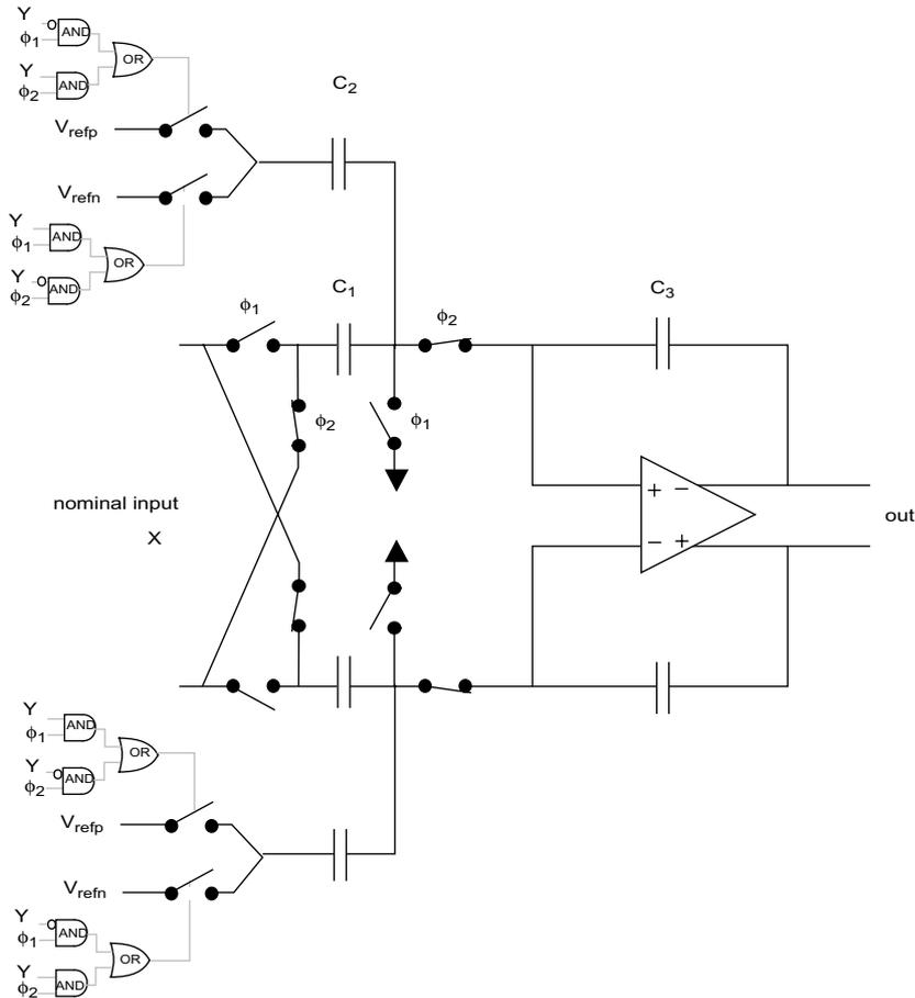
**Figure 6-23: Two-branch integrator with double-sampling on both branches**
