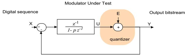
Figure 4-6: z-domain representation of a linearized first-order multibit  $\Sigma\Delta$  modulator
