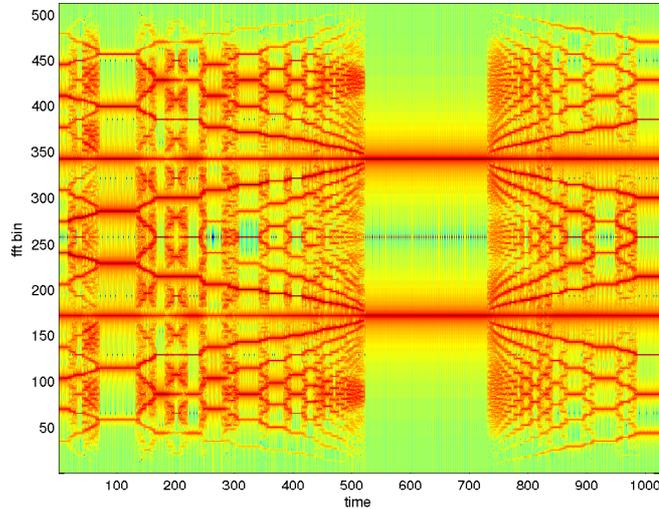
**Figure 4-17: Evolution in time of the output bitstream spectrum for a [1 1 -1] input sequence**
