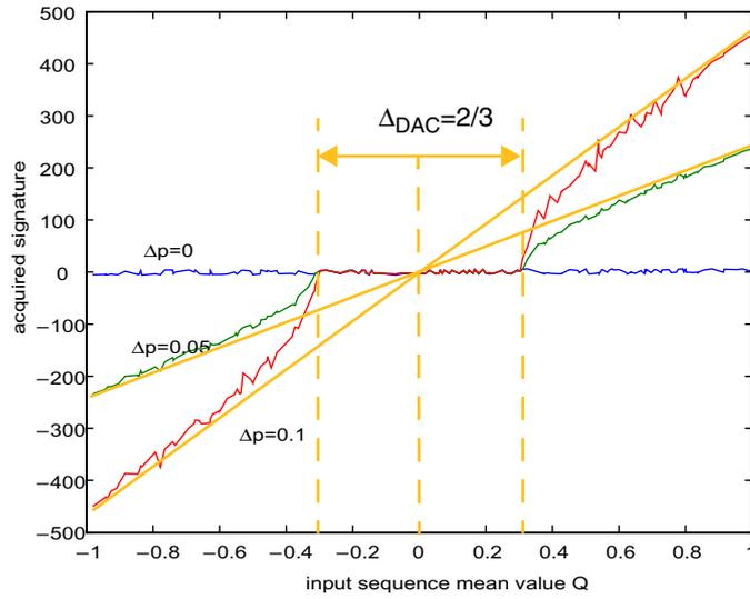
**Figure 4-19:** Test signature output as a function of the input sequence mean value, for a 2-bit modulator
