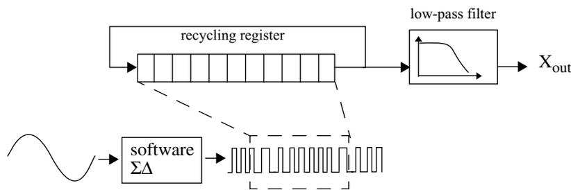
**Figure 2-3:** A  $\Sigma\Delta$  programmable periodic wave
