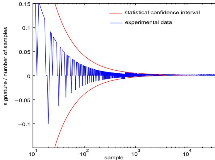
**Figure 7-27:** Evolution of the 2<sup>nd</sup> integrator leakage signature as function of the number of points
