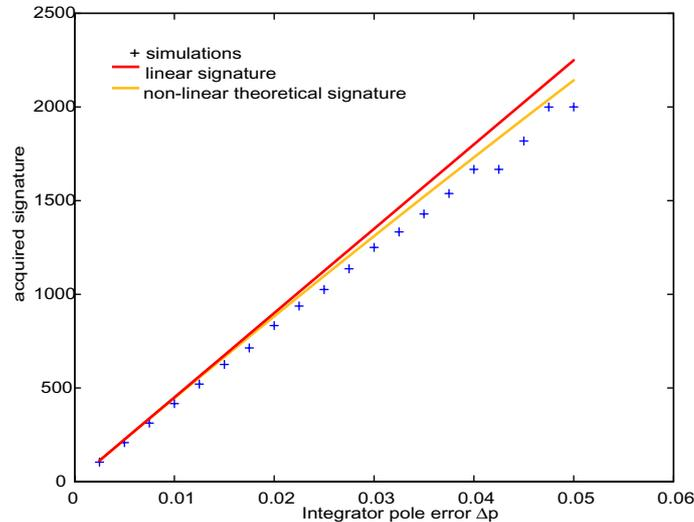
**Figure 4-22:** Test signature output as a function of the integrator leakage ( $\Delta p$ ) for a 2-bit first-order modulator
