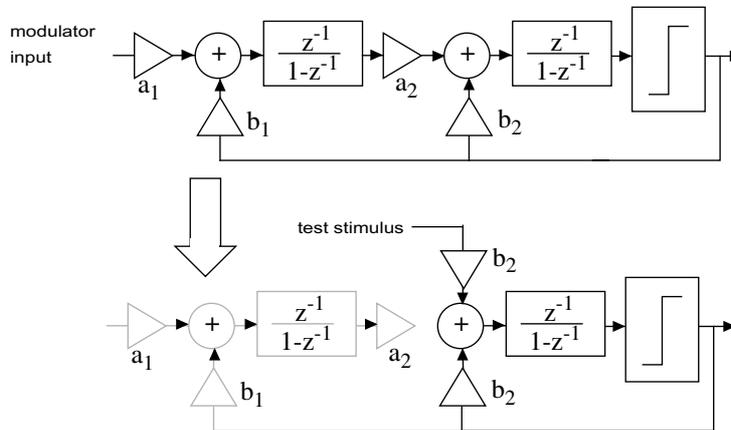
**Figure 3-8: Reconfiguration of a 2nd order modulator as a 1st order modulator, for test purpose**
