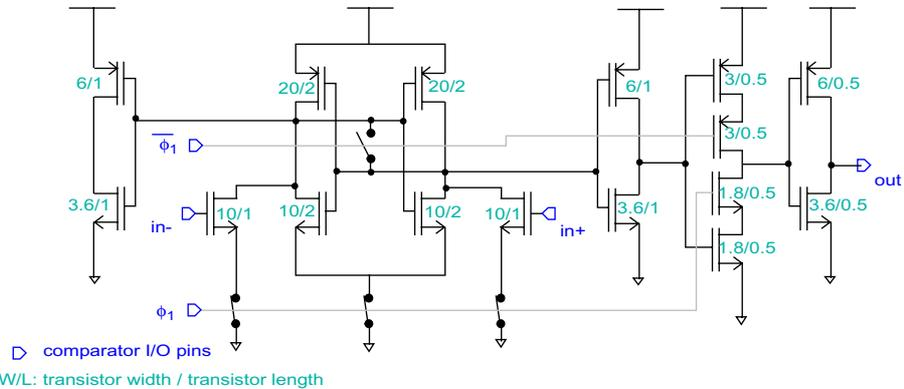
**Figure 7-8: Comparator schematics**
