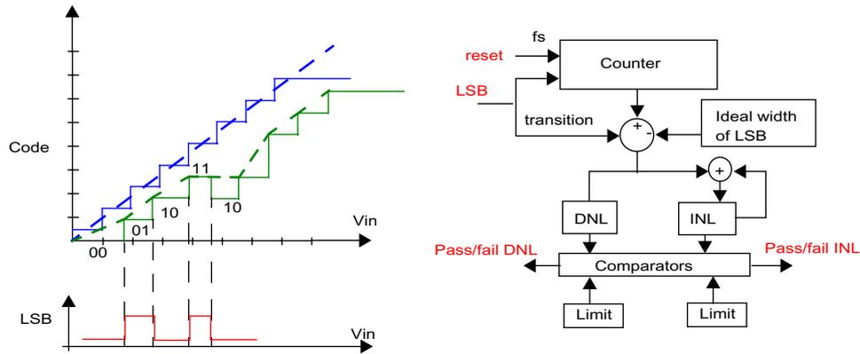
**Figure 2-7: On-chip INL and DNL checking by monitoring LSB**
