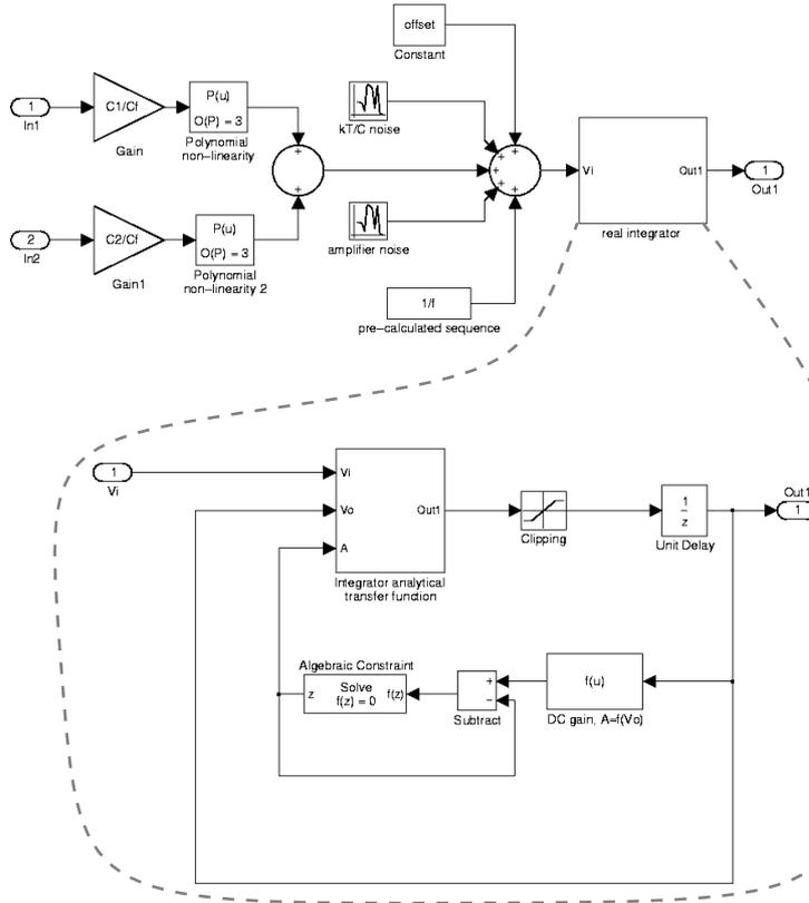
**Figure 1-13: Simulink model of a two branch integrator**
