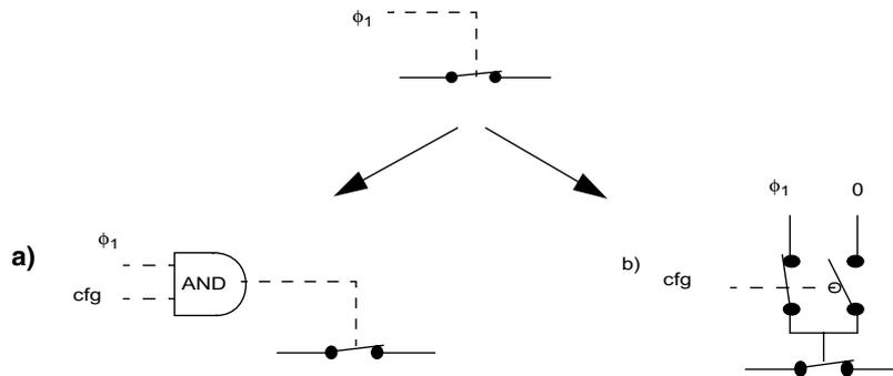
**Figure 6-17: Integrator input switch - control modification.**
