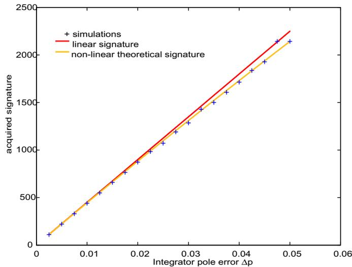
**Figure 4-21: Test signature output as a function of the integrator leakage ( $\Delta p$ ) for a 3-bit first-order modulator**
