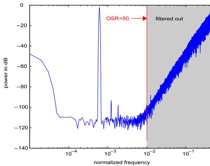
**Figure 7-20:** Nominal  $\Sigma\Delta$  output spectrum for a  $550\text{mV}_{\text{rms}}$  input sine-wave (i.e. 78% of full-scale)
