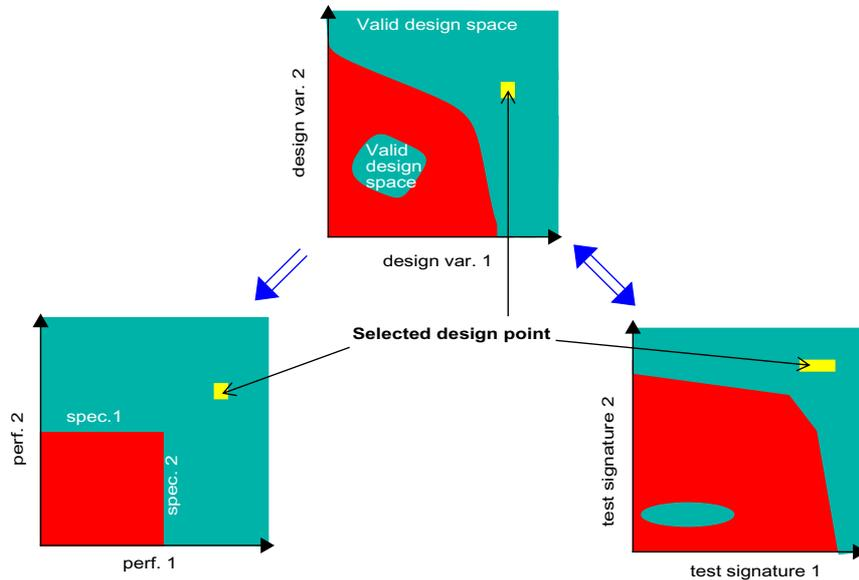
**Figure 3-2:** Relation between design space, performance space and test signature space
