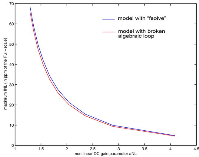
Figure 1-15: Maximum INL of a 2<sup>nd</sup> order modulator as function of the 1<sup>st</sup> amplifier DC gain non-linearity
