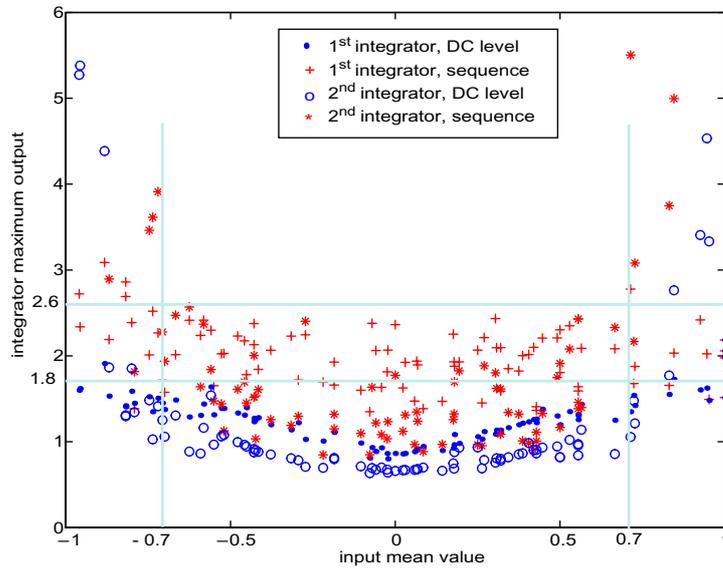
Figure 6-1: Maximum integrator outputs as a function of modulator A input
