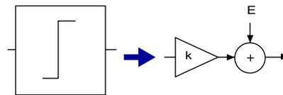
Figure 4-5: Quantizer linear model
