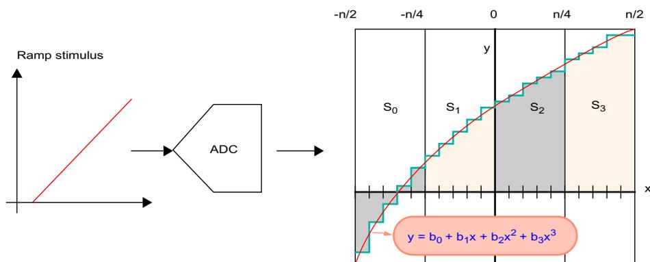
**Figure 2-10:** Test with a 3rd order polynomial model
