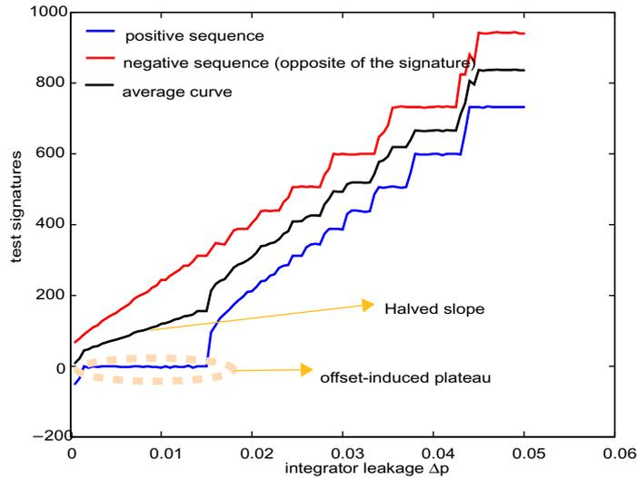
**Figure 4-30:** Test signature versus integrator leakage, for an input sequence of  $L=6$  and its opposite, and an input-referred offset of 0.003.
