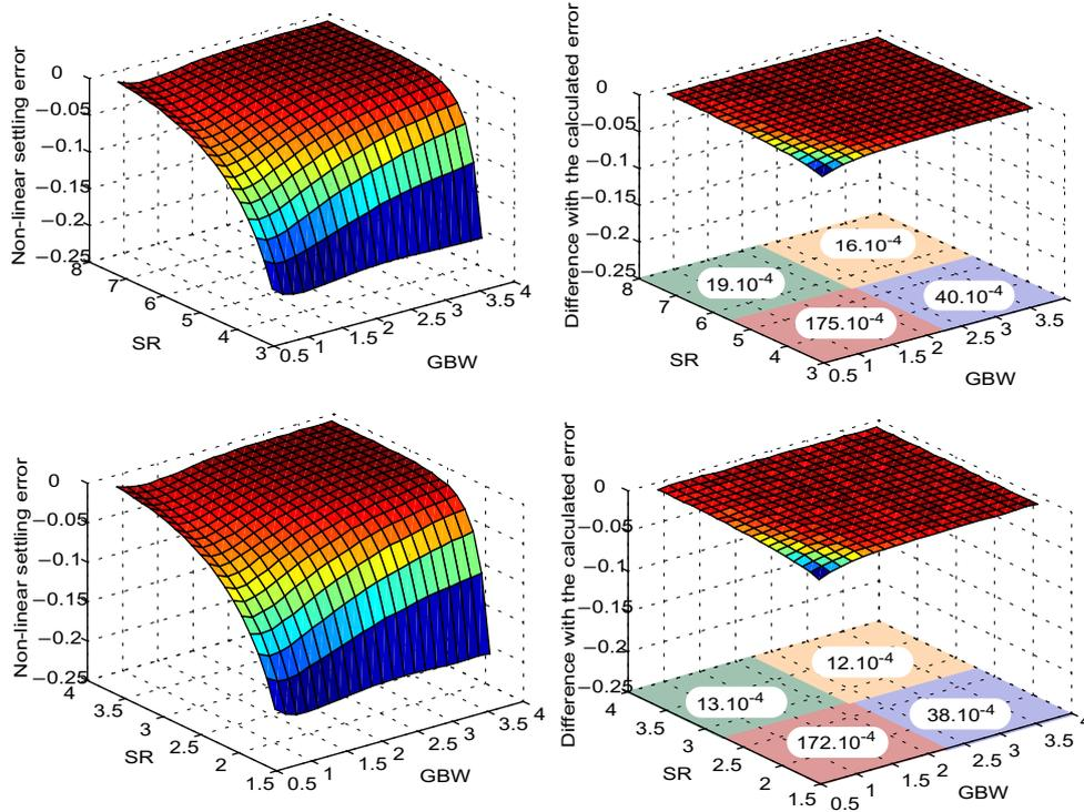
**Figure 5-18: Evaluated non-linear settling error and its difference with the calculated non-linear settling error**
