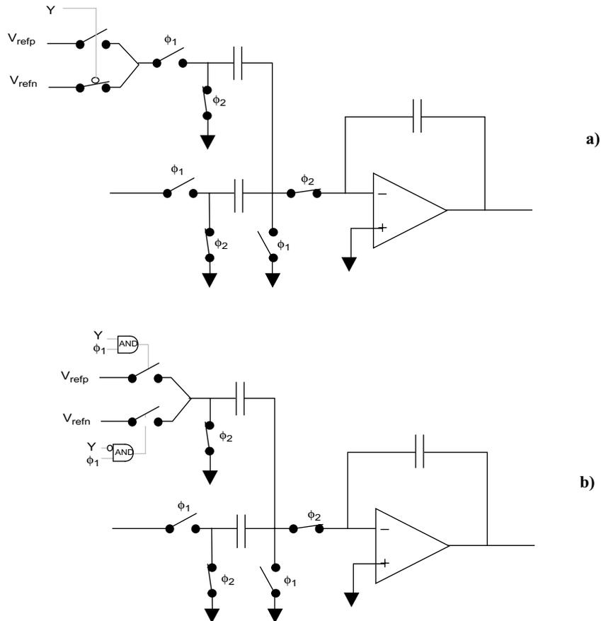
**Figure 6-20: a) direct connection of the feedback DAC to the integrator
