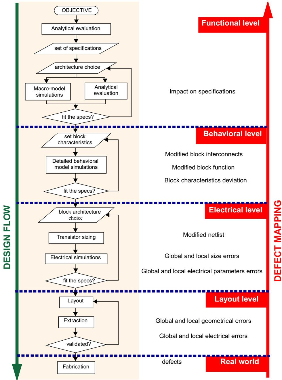
Figure I-2: Relating design-flow and defect mapping
