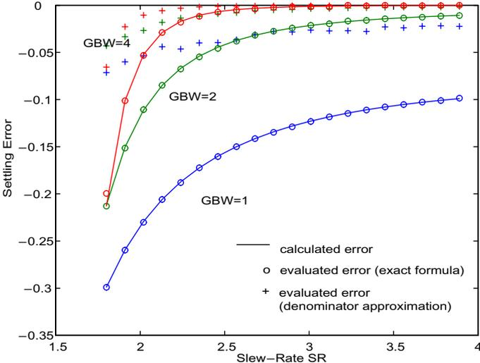
Figure 5-13: Second order modulator settling error evaluation for a [1 -1] input sequence.
