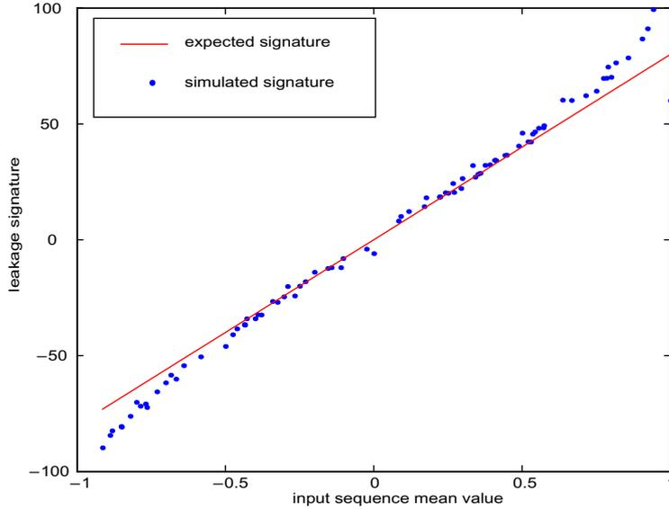
**Figure 6-3: Modulator A 1<sup>st</sup> integrator leakage signature as a function of the mean value of the input sequence**
