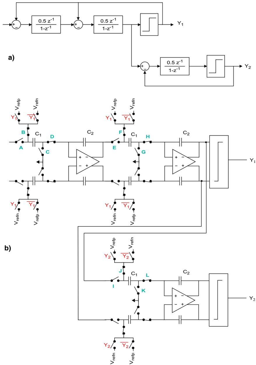
**Figure 7-1:** 2-1 cascaded  $\Sigma\Delta$  modulator
