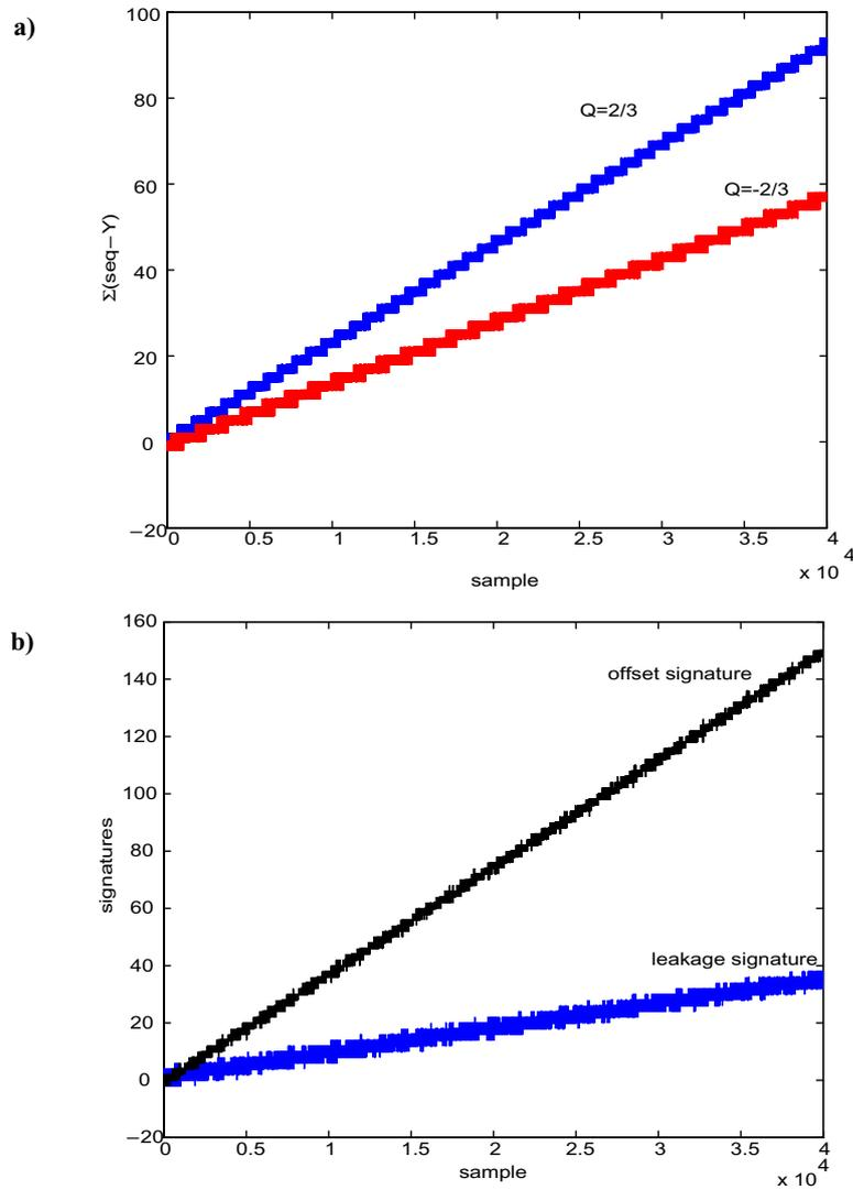
**Figure 7-22: Evolution with time for the leakage test of the first integrator**
