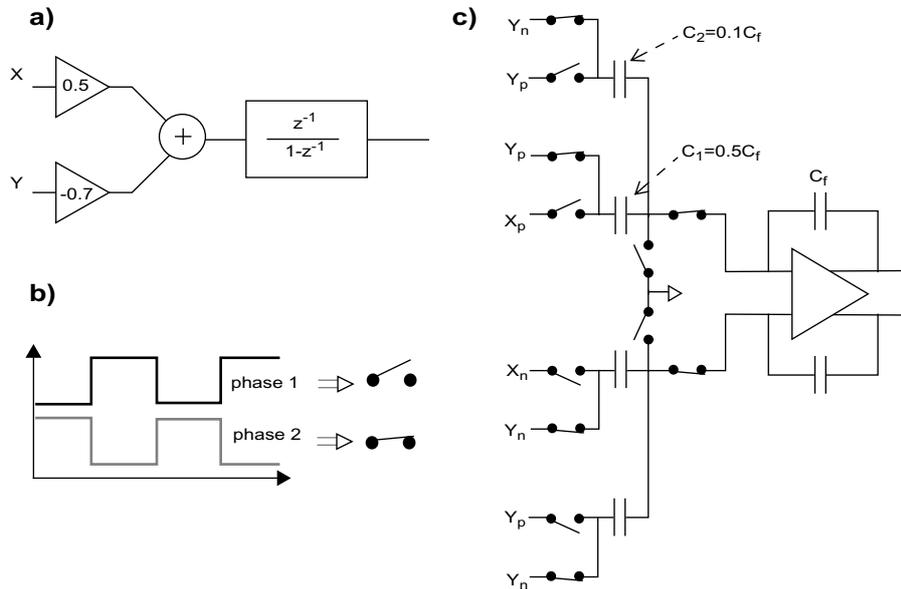
**Figure 1-11:** a) z-domain model of a two-branch integrator; b) non-overlapping phases; c) possible switched-capacitor implementation.
