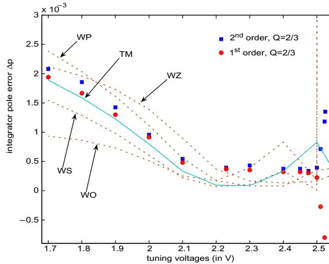
**Figure 7-28: Integrator leakage as function of the tuning voltage**
