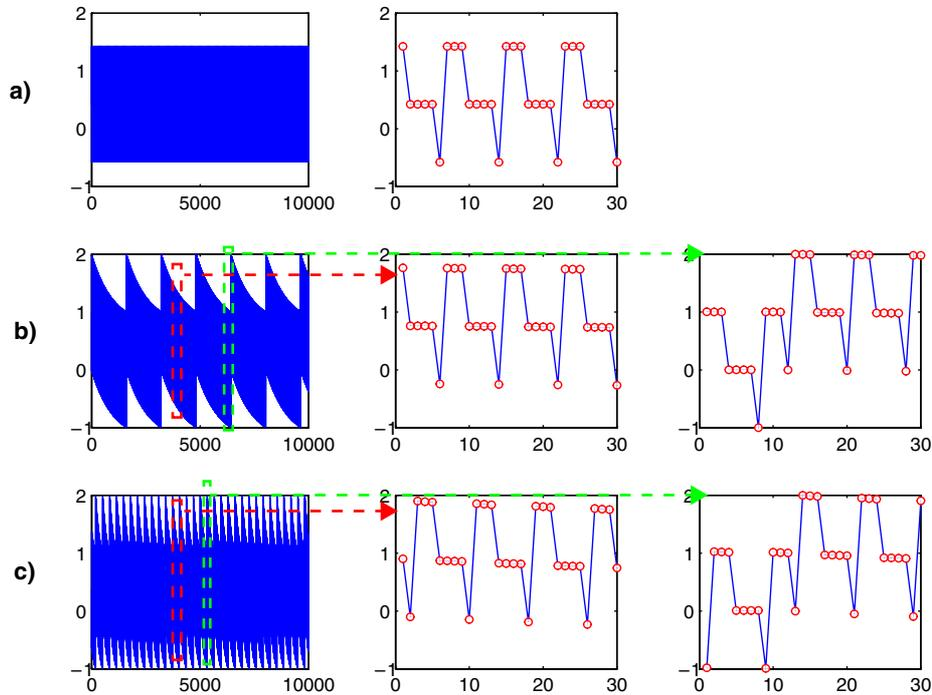
**Figure 4-32:** Integrator output, for a 1<sup>st</sup> order single-bit modulator.
