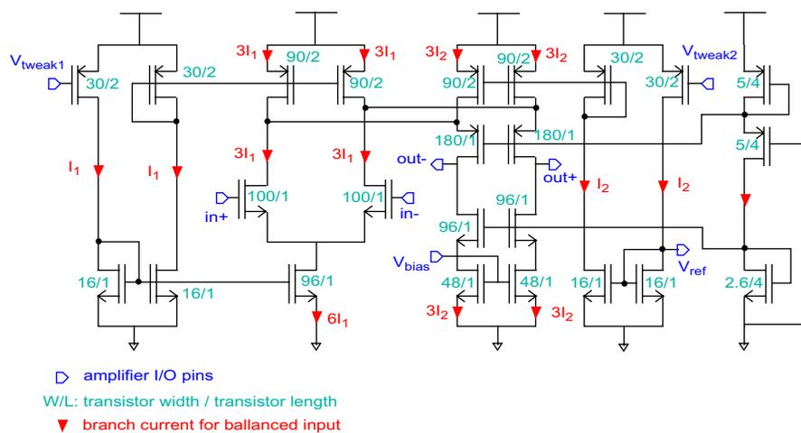
**Figure 7-2: Schematics of the amplifier with parametric fault injection mechanism through  $V_{tweak1}$  and  $V_{tweak2}$**
