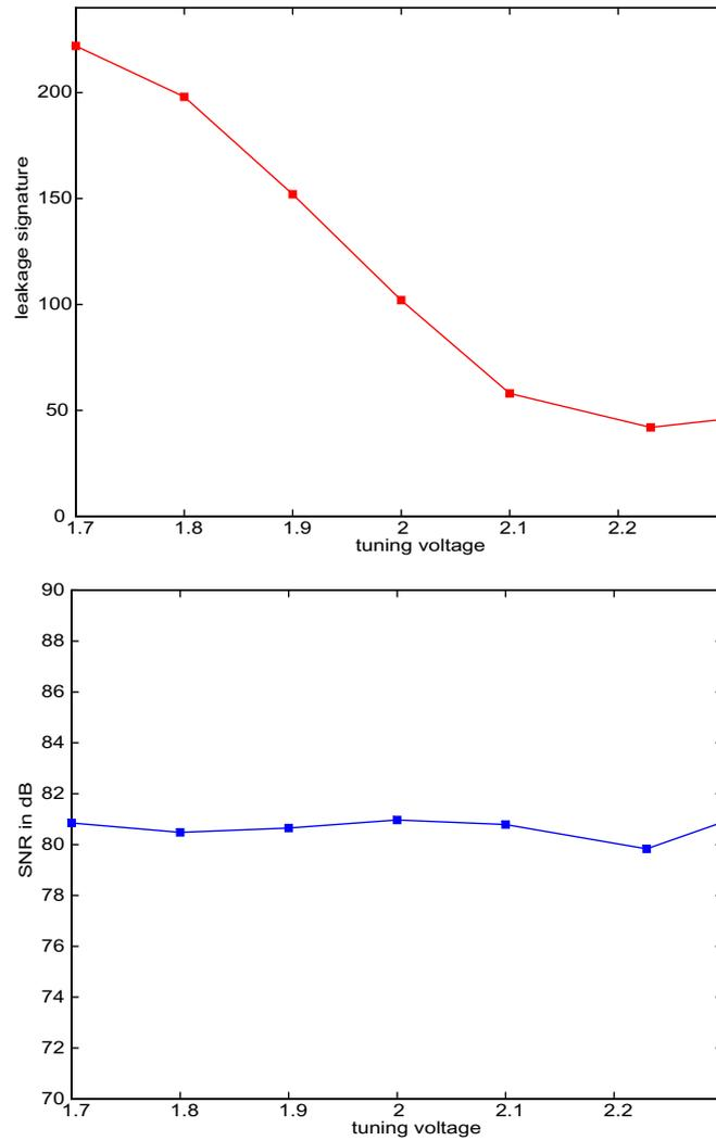
**Figure 7-29: Correlation between the first integrator leakage signature and the measured modulator SNR**
