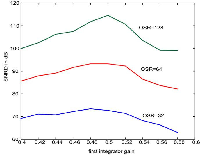
**Figure 5-3: SNRD of a 2-1 cascaded modulator versus its first integrator gain**
