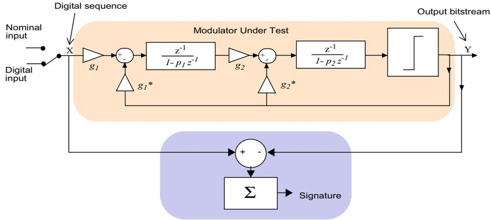
**Figure 4-3: Diagram of the proposed test for first integrator leakage in a second-order  $\Sigma\Delta$  modulator**
