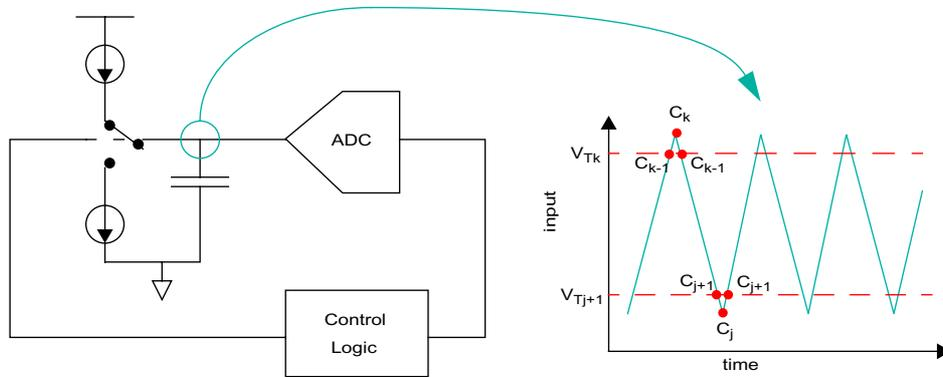
**Figure 2-9: A BIST application of the servo-loop principles**
