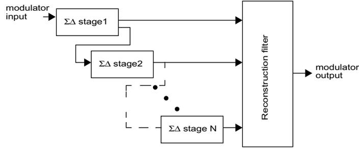
**Figure 1-10: Diagram of cascaded  $\Sigma\Delta$  modulators**
