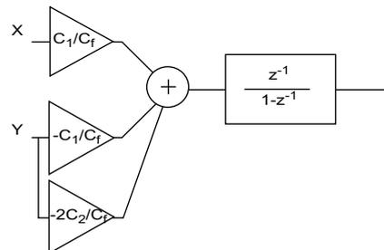
**Figure 1-12:** Good parametrization of the integrator z-domain model
