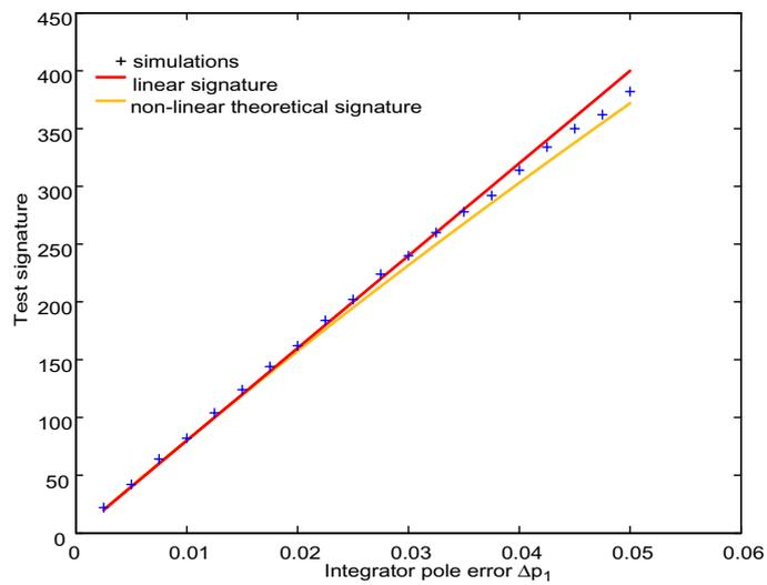
**Figure 4-16:** Test signature output as a function of the first integrator leakage ( $\Delta p_2=0.05$ )
