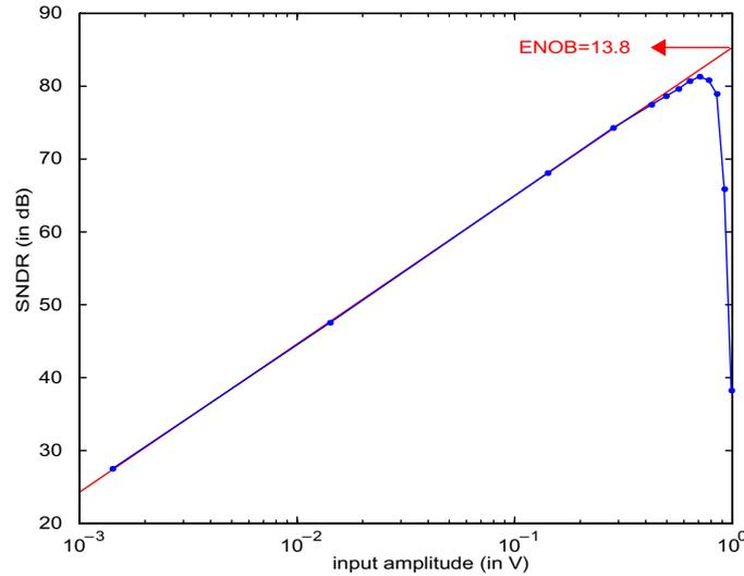
**Figure 7-18: SNDR versus input sine-wave amplitude, for an OSR of 50**
