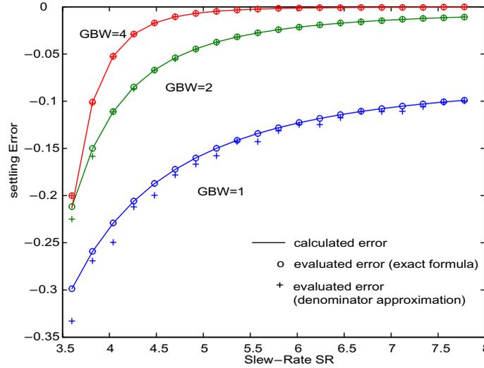
**Figure 5-10: First order modulator settling error evaluation for a [1 1 -1 1 -1 -1] input sequence.**
