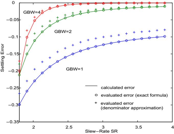
Figure 5-14: Second order modulator settling error evaluation for a [1 1 -1 -1 -1] input sequence.
