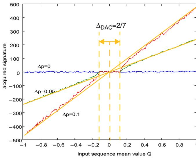
**Figure 4-20:** Test signature output as a function of the input sequence mean value, for a 3-bit modulator
