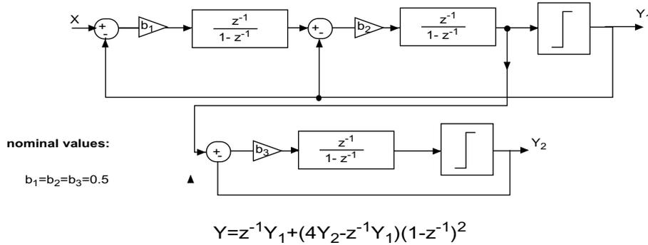
**Figure 5-2: Diagram of a 2-1 cascade modulator**
