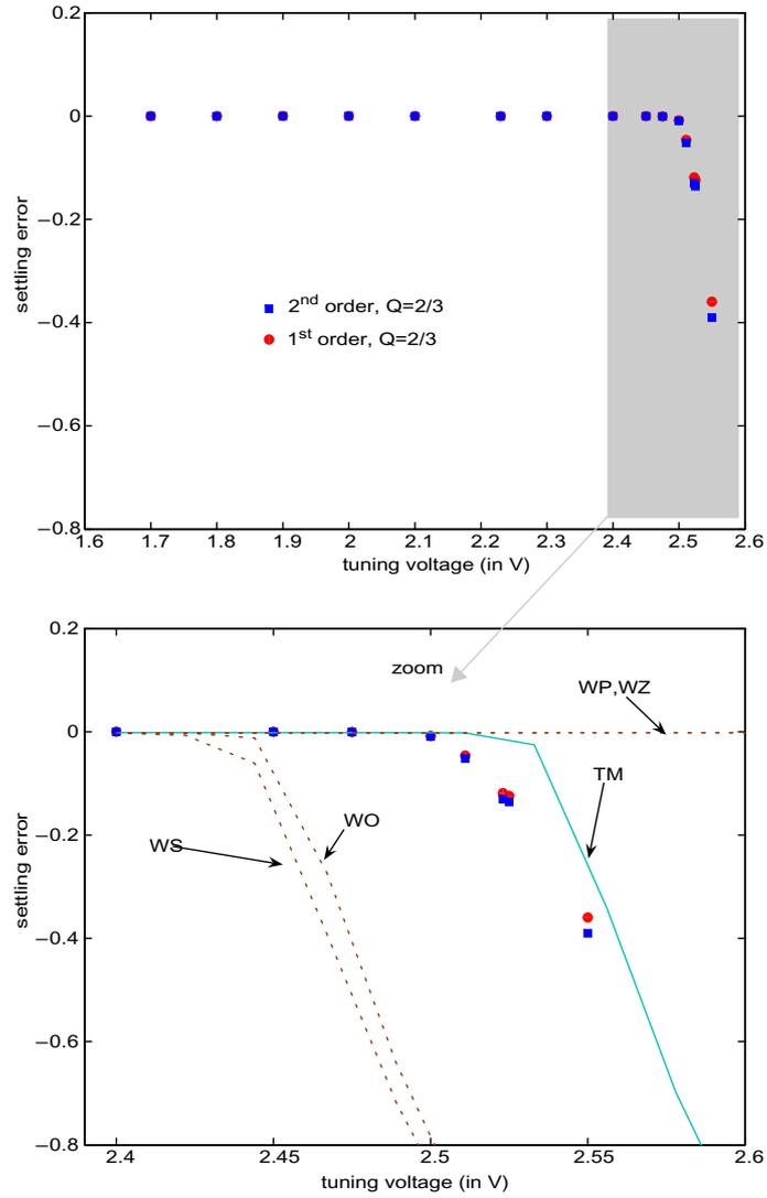
**Figure 7-35: Measured (markers) and simulated (solid and dashed curves) settling errors**
