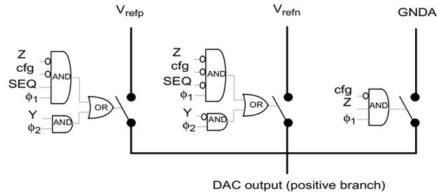
**Figure 6-27:** Example of implementation of a 3-level test DAC
