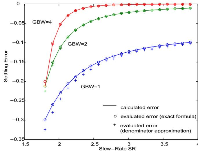
**Figure 5-15:** Second order modulator settling error evaluation for a random input sequence.
