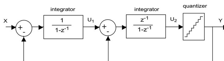
**Figure 1-7: Stable double-loop 2<sup>nd</sup> order  $\Sigma\Delta$  modulator**
