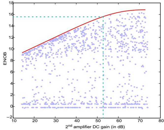
**Figure 5-21:** Cloud of points of the design space exploration representing the obtained ENOB versus the 2nd amplifier DC gain
