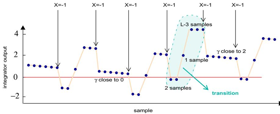
**Figure 4-10: Transition pattern for the case of a leaky integrator**
