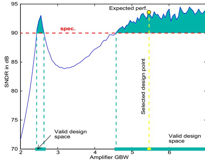
**Figure 3-3:** Impact of 1<sup>st</sup> amplifier Gain-Bandwidth product on the SNDR of a 2-1 cascaded  $\Sigma\Delta$  modulator
