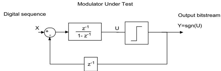
**Figure 4-7: z-domain representation of a first-order single-bit  $\Sigma\Delta$  modulator with an extra delay in the feedback path.**
