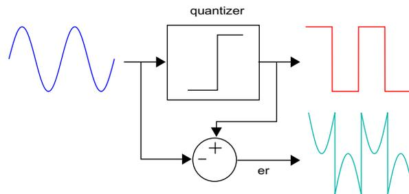
**Figure 1-4:** 1-bit quantizer error
