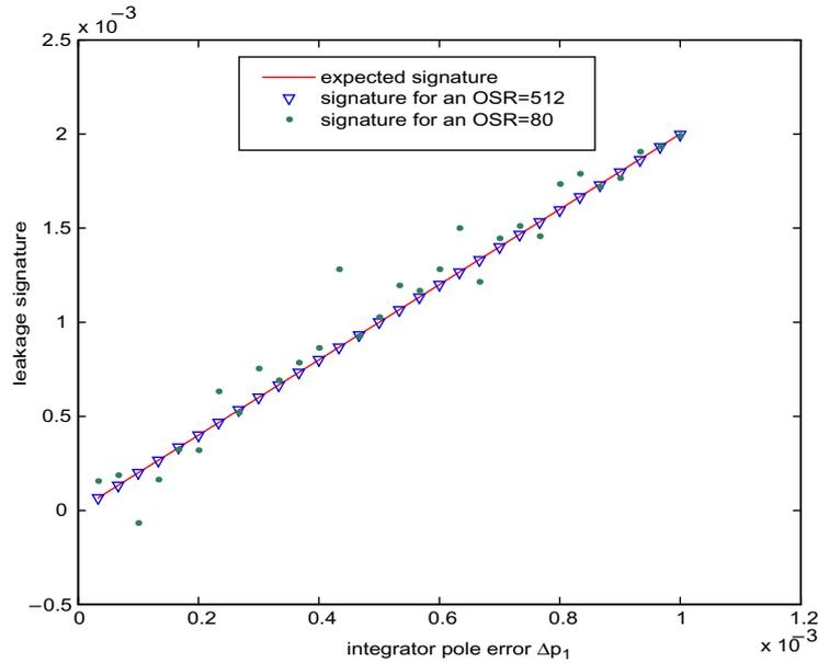
**Figure 6-15: Leakage test signature for two OSR values**
