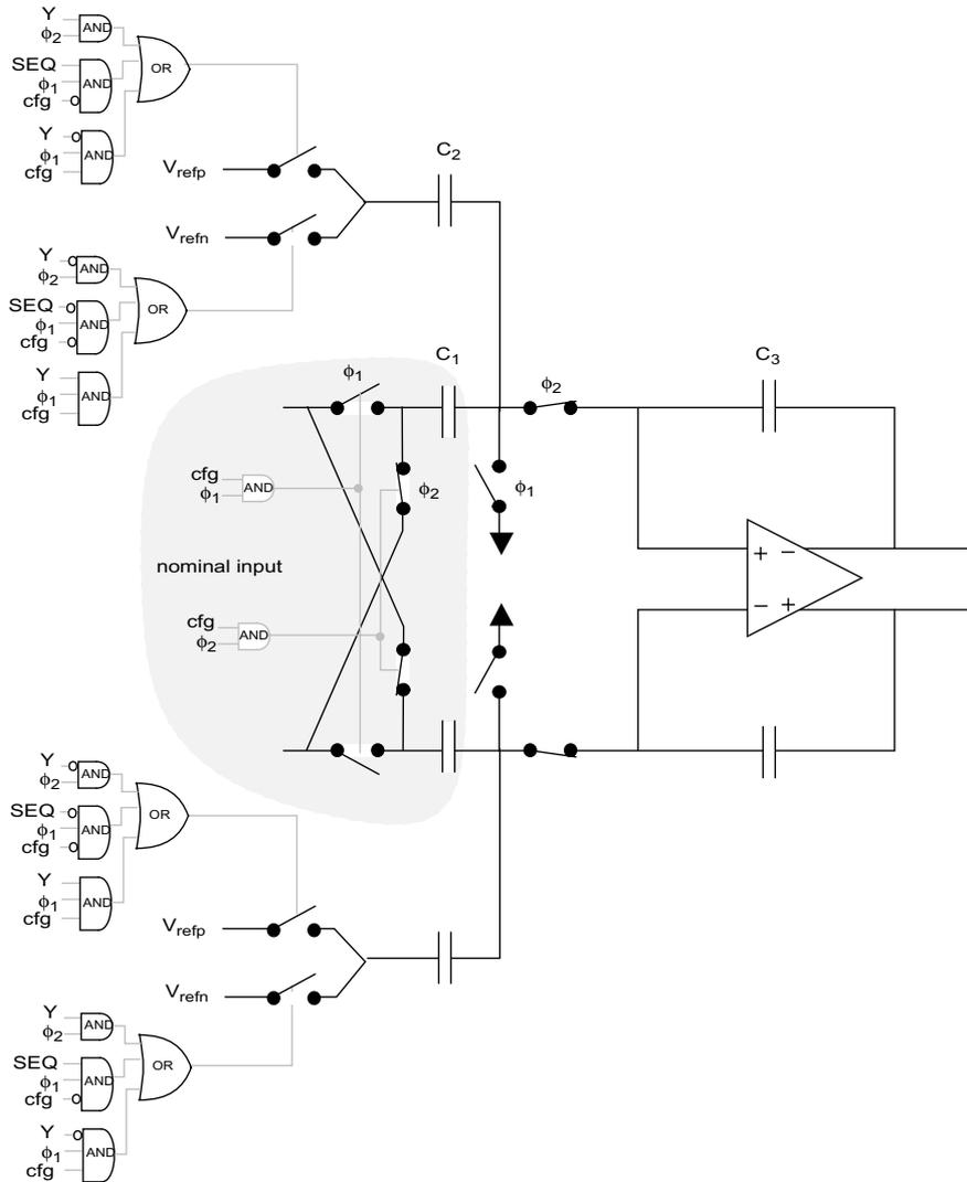
**Figure 6-24:** Disabling double-sampling to input a digital sequence
