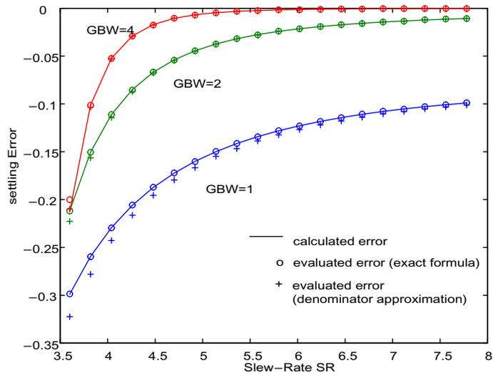
Figure 5-12: First order modulator settling error evaluation for a random input sequence.
