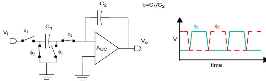
**Figure 5-1: Switched-capacitor integrator scheme**
