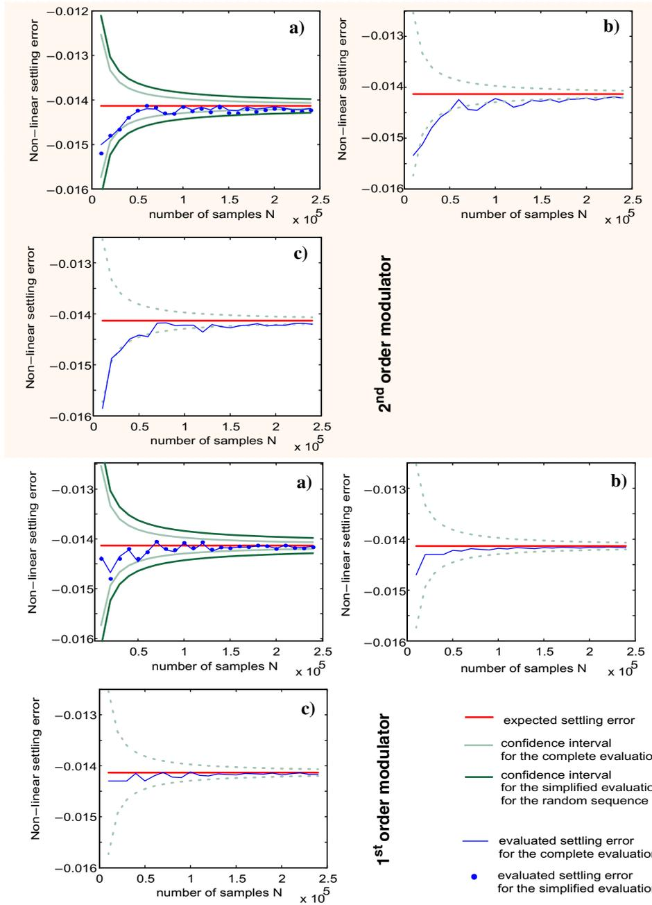
**Figure 5-19: First and second order modulator settling error evaluation versus the number of acquired points**
