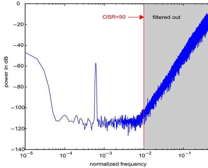
**Figure 7-19:** Nominal  $\Sigma\Delta$  output spectrum for a  $1\text{mV}_{\text{rms}}$  input sine-wave
