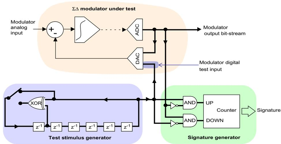
**Figure 3-5:** Generic scheme of the proposed test setup
