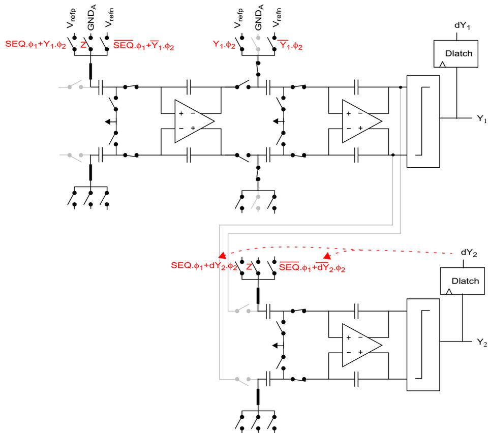
**Figure 7-15:** The  $\Sigma\Delta$  modulator reconfigured to test the leakage of the 1<sup>st</sup> and 3<sup>rd</sup> integrators in parallel
