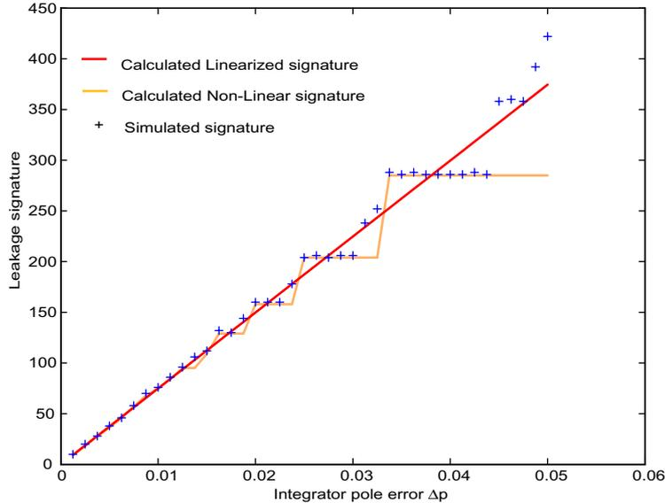
**Figure 4-35: Alternative test signature versus integrator leakage, for an input sequence of  $L=7$**
