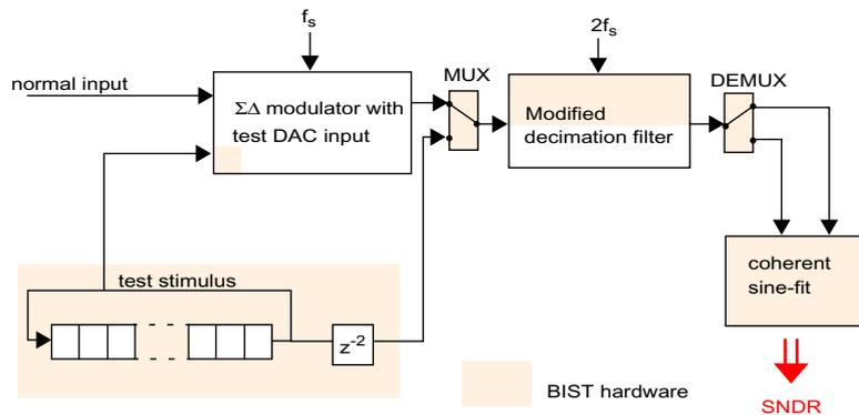
**Figure 2-13:** Digital sine-fit BIST setup
