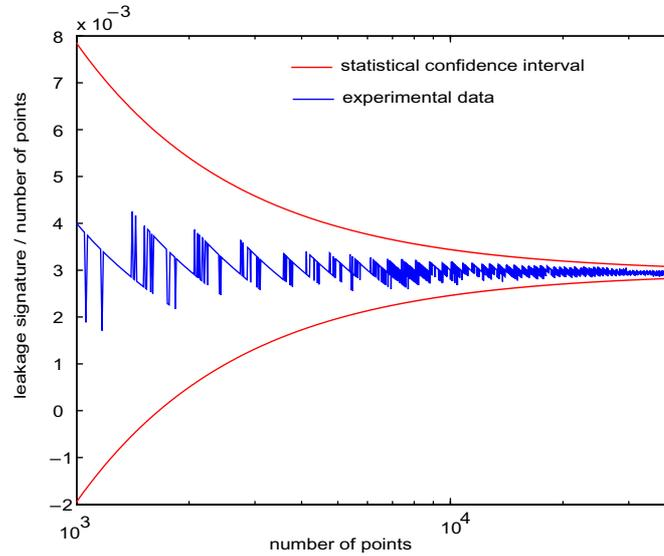
**Figure 7-26:** Evolution of the 1<sup>st</sup> integrator leakage signature as function of the number of points
