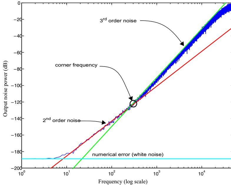
**Figure 4-2: Output noise spectrum of a 3rd order  $\Sigma\Delta$  modulator with a leaky integrator**
