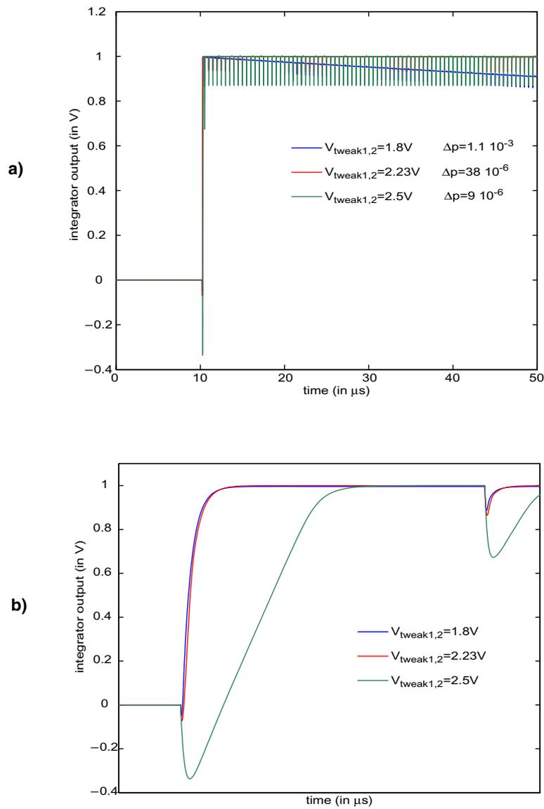
**Figure 7-6:** Integrator response to an input pulse, for 3 values of the tuning voltages
