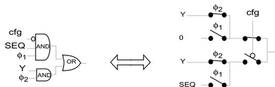
**Figure 6-26:** Implementation of DAC control with transmission gates
