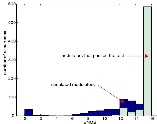
**Figure 5-27:** Histograms of the ENOB obtained for the 1000 simulated modulators and for the subset of the modulators that passed the test set with performance-oriented limits
