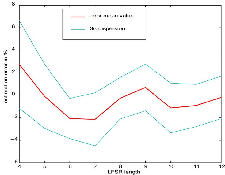
**Figure 6-11:** Estimation error of the number of occurrences of level 2, as a function of the LFSR length
