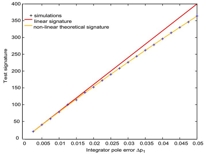
**Figure 4-15:** Test signature output as a function of the first integrator leakage ( $\Delta p_2=0$ )
