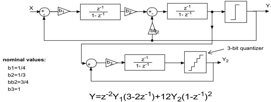
Figure 5-20: Diagram of a 2-1 cascade modulator
