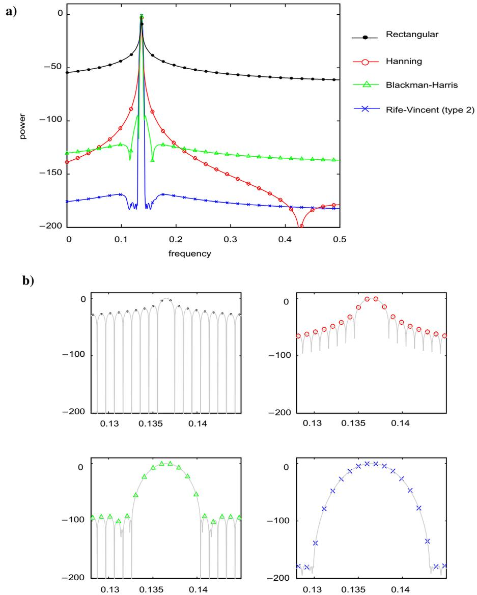
**Figure 1-23:** a) 1024 points FFT of four windows in the worst case of non-coherent sampling (signal between two FFT bins) b) Main lobes of the window spectra
