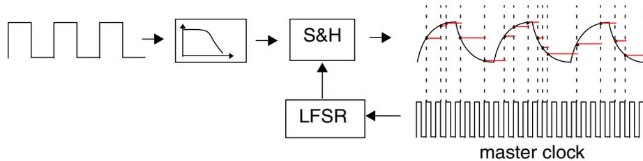
**Figure 2-5: Noise generator based on a statistical sampler**
