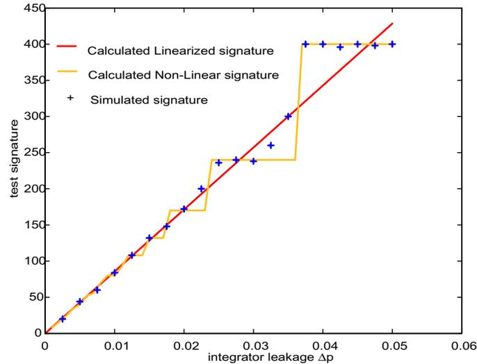
**Figure 4-28:** Test signature versus integrator leakage, for an input sequence of  $L=11$
