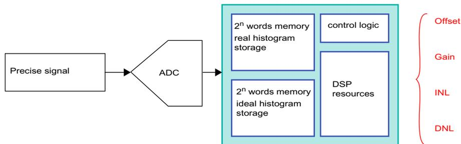
**Figure 2-8: Generic hardware required to perform an histogram test**
