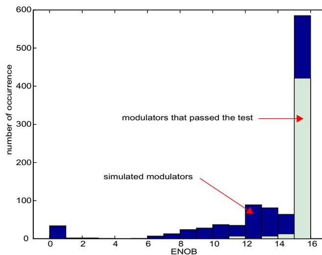
**Figure 5-26:** Histograms of the ENOB obtained for the 1000 simulated modulators and for the subset of the modulators that passed the test set
