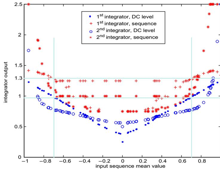
**Figure 6-7:** Maximum integrator outputs as a function of the modified modulator A input
