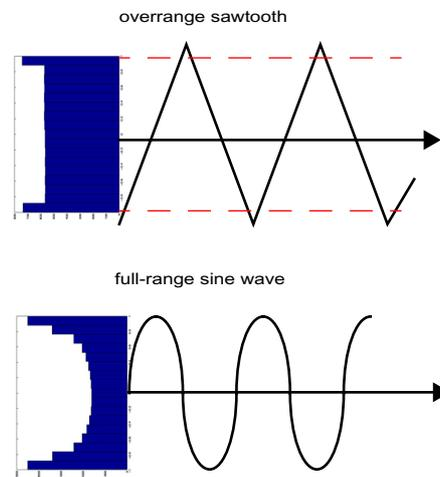
**Figure 1-21: Sawtooth and sine-wave density histograms**
