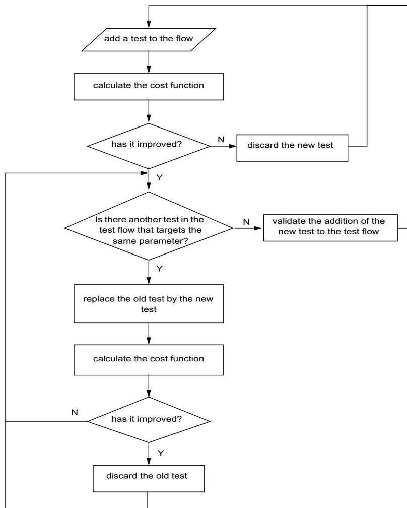
**Figure 5-24:** Ad-hoc test flow optimization algorithm
