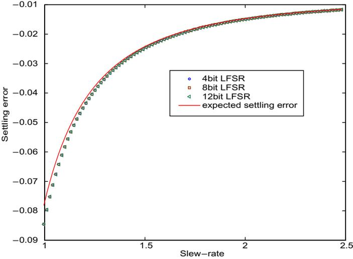
**Figure 6-6:** Modulator B settling error signature as a function of the 1st integrator Slew-rate.
