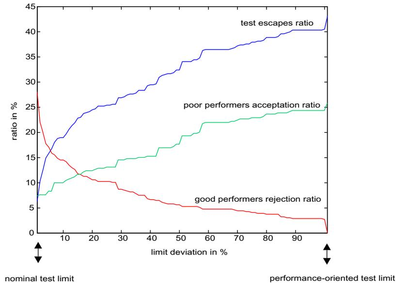
**Figure 5-28: Evolution of two test metrics as function of the test limits:**
