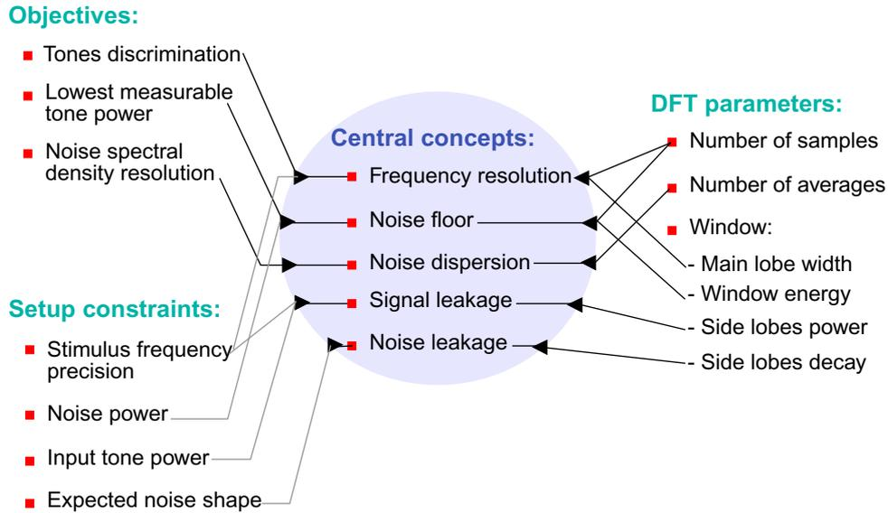
**Figure 1-24: Relating FFT parameters to test objectives and setup constraints**
