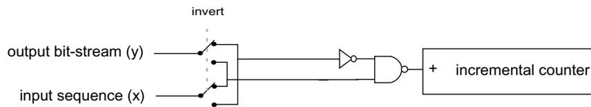
**Figure 6-14: Counter of level 2 (-2) number of occurrences at the integrator input**
