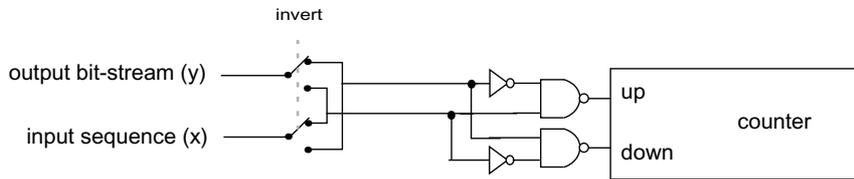
**Figure 6-13: Hardware required for the signatures**
