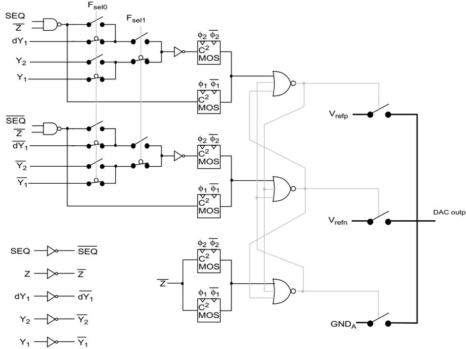
**Figure 7-11: Positive branch of the DAC modified for test purpose**
