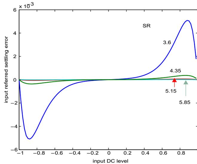
**Figure 5-5: Input referred settling error versus DC input level (normalized to Full-Scale)**
