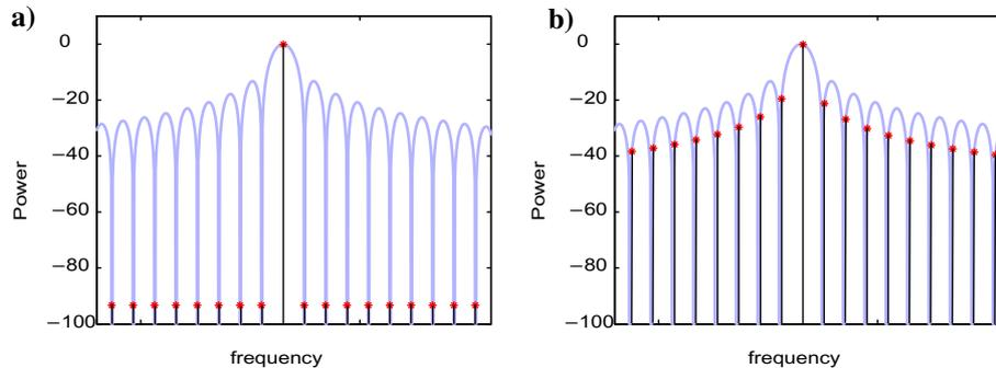
**Figure 1-22: Spectrum of a rectangular window. a) for a coherent tone, b) for a non-coherent tone**
