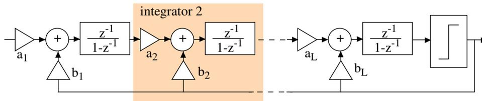
**Figure 3-6:** Direct extension of the feedback structure to modulators of order higher than 2
