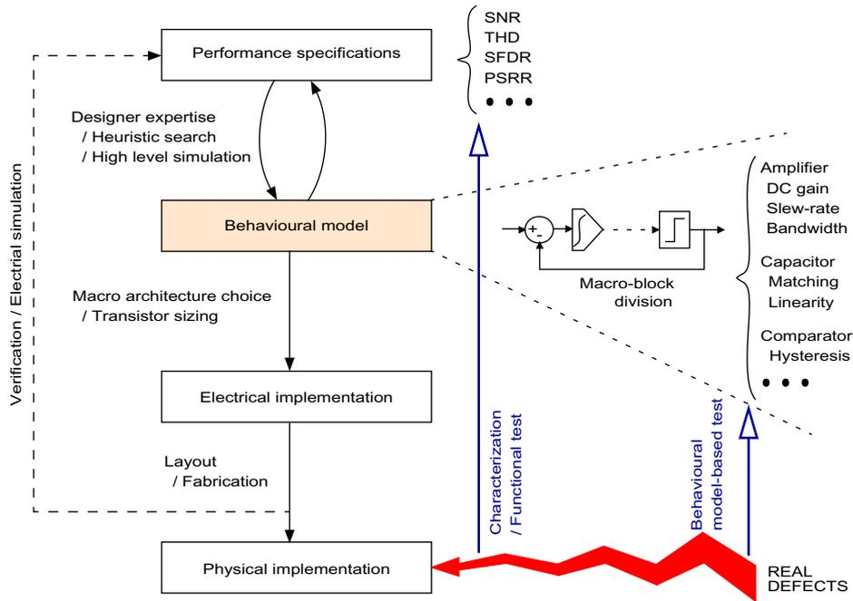
**Figure 3-1: Behavioural model in the design and test flow**
