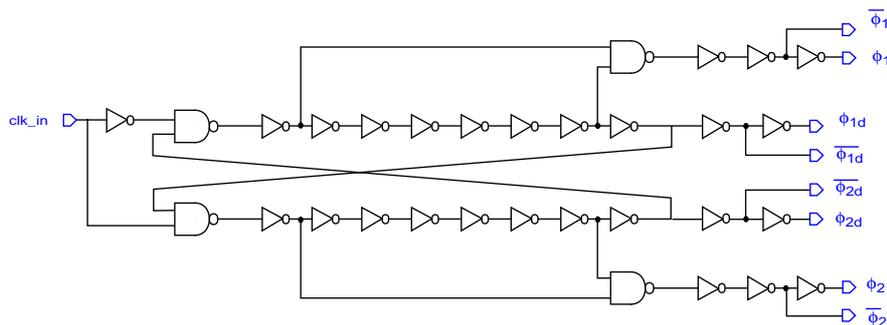
**Figure 7-7: Non-overlapping phase generator**
