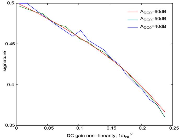
**Figure 4-39:** Proposed test signature as function of the DC gain non-linear parameter  $a_{NL}$  for 3 values of the nominal DC gain.
