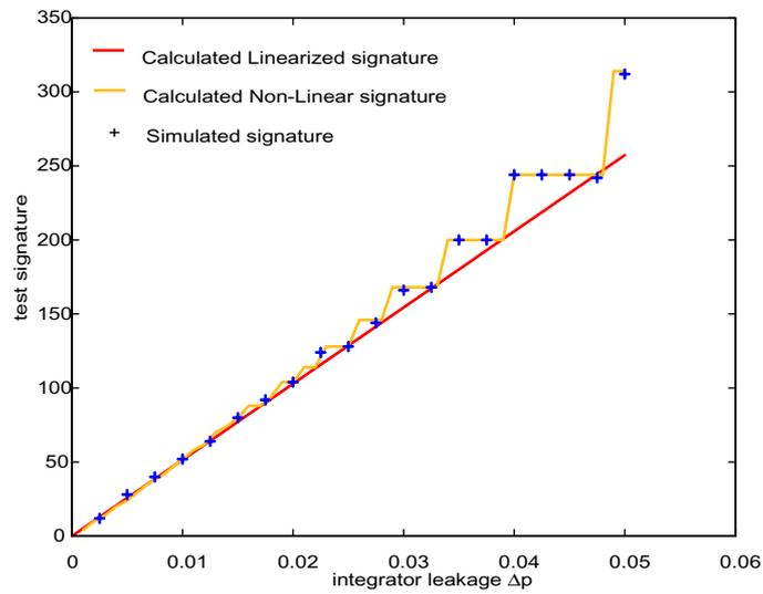
**Figure 4-27:** Test signature versus integrator leakage, for an input sequence of L=6
