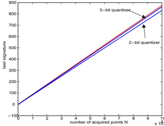
**Figure 4-23:** Test signature as a function of the number of acquired points for a 3-bit quantizer and a 2-bit quantizer
