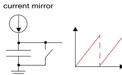
**Figure 2-4: Generic scheme of a ramp generator**
