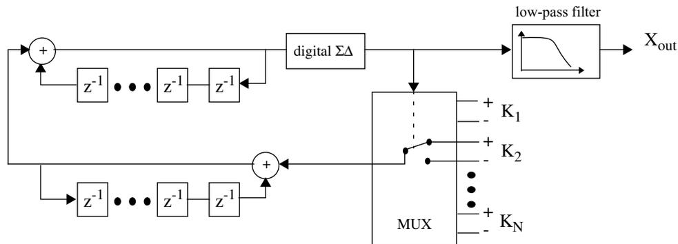
**Figure 2-2:** A  $\Sigma\Delta$  oscillator with programmable frequency
