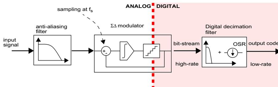
**Figure 1-1:** The structure of a  $\Sigma\Delta$  converter
