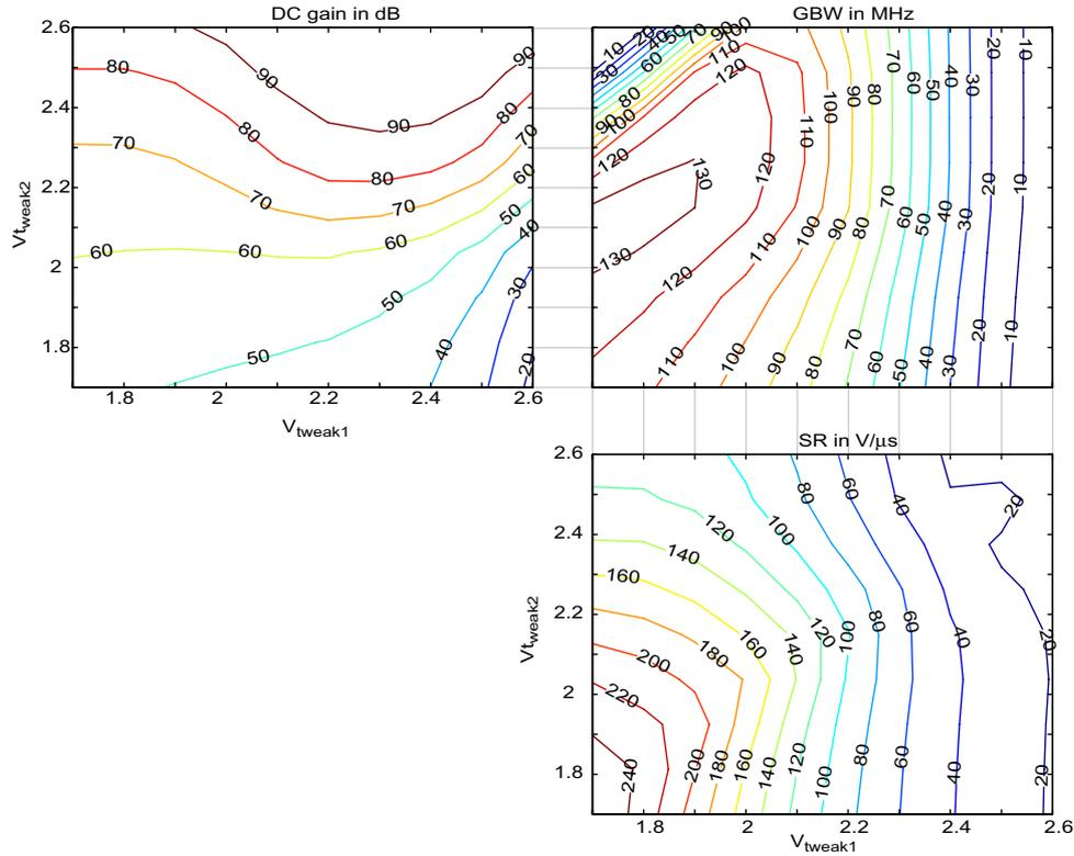
Figure 7-3: Iso-levels of amplifier parameters when varying the two tuning inputs
