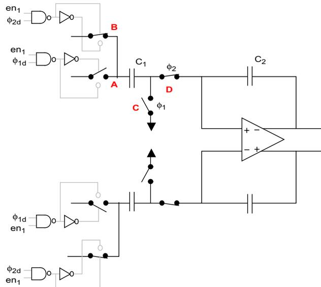
**Figure 7-10: Modification of the integrator switch control to enable the test input**
