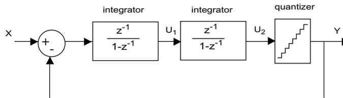
**Figure 1-6: Direct unstable implementation of a 2<sup>nd</sup> order  $\Sigma\Delta$  modulator**
