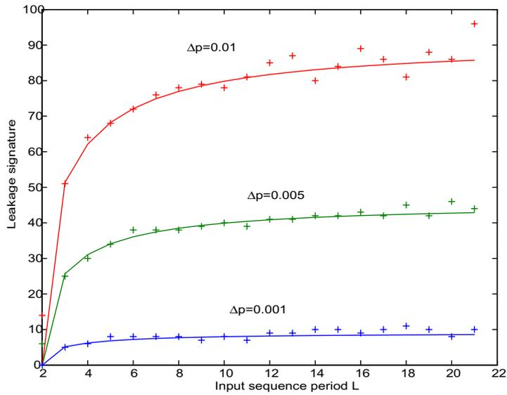
**Figure 4-33:** Alternative test signature versus test sequence period L, for a 1st order single-bit modulator.
