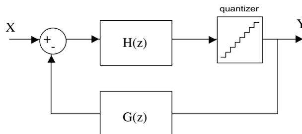
**Figure 1-8: Generalized  $\Sigma\Delta$  modulator diagram**
