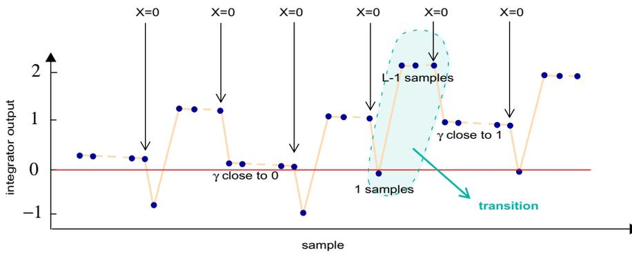
Figure 4-13: Transition pattern at the integrator output for a leaky integrator
