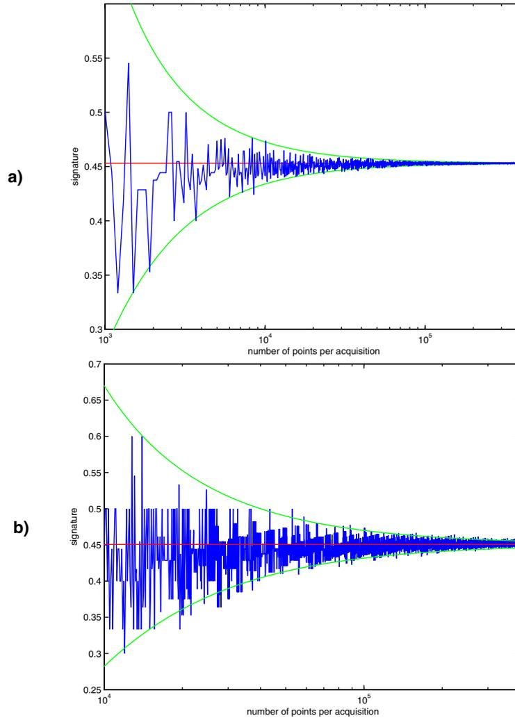
**Figure 4-40: Proposed test signature as a function of the number of acquired points.**
