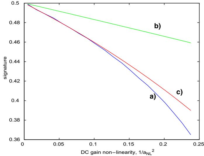
**Figure 4-41:** Proposed test signature as function of the DC gain non-linear parameter  $a_{NL}$
