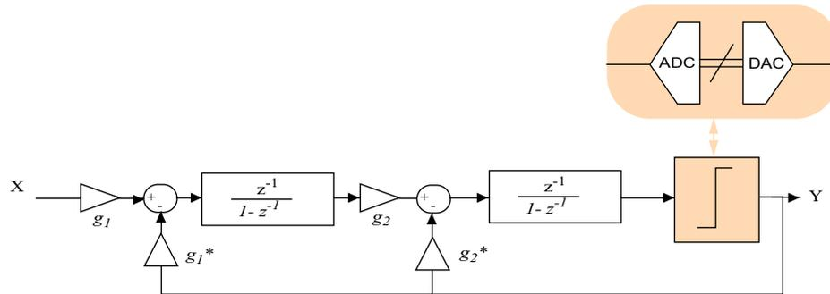
**Figure 3-9: Discrete-time representation of a 2nd order  $\Sigma\Delta$  modulator**
