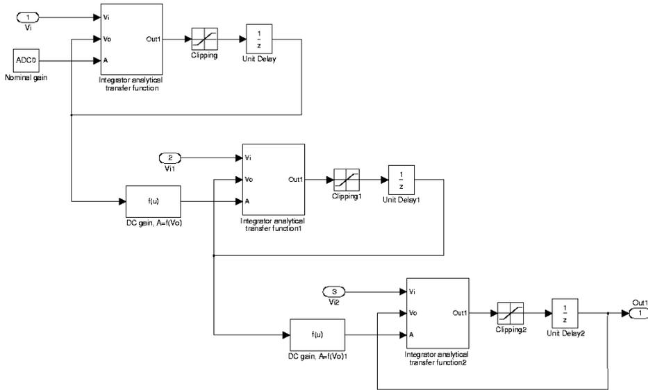
Figure 1-14: Opening the algebraic loop
