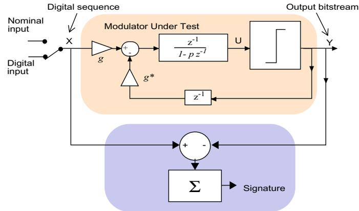
**Figure 4-4:** Diagram of the proposed test for first integrator leakage in a first-order single-bit  $\Sigma\Delta$  modulator
