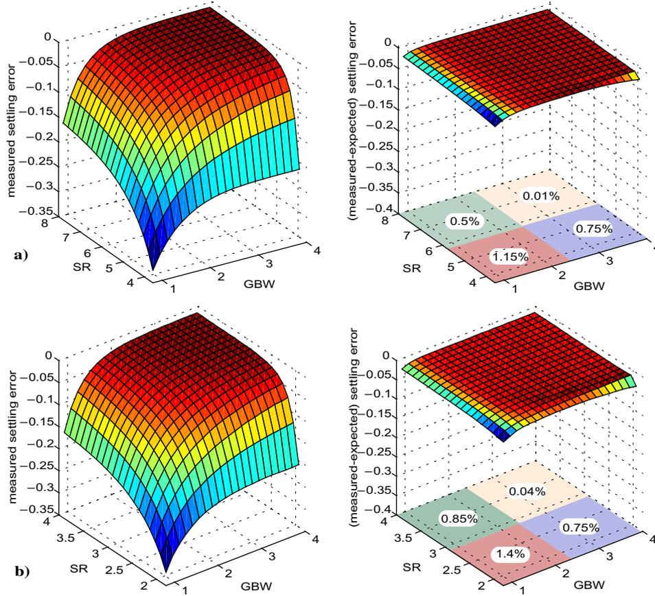
**Figure 5-8: Evaluated settling error and its difference with the calculated settling error**
