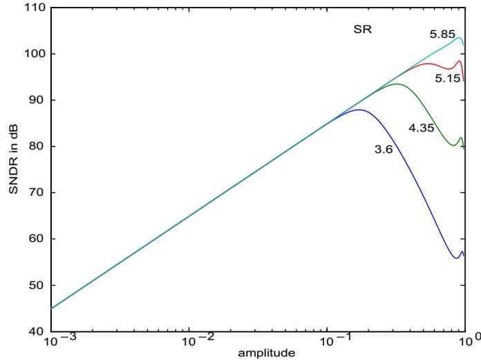
**Figure 5-4: SNDR versus input sinewave amplitude, for different values of SR**
