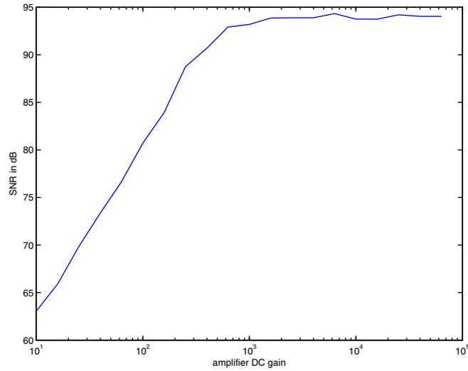
**Figure 1-16: SNR of a 2-1 cascaded modulator as function of the 1<sup>st</sup> amplifier DC gain**
