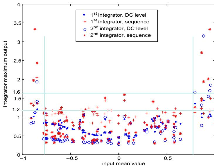
Figure 6-2: Maximum integrator outputs as a function of modulator B input
