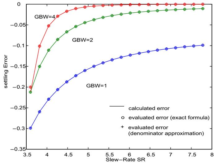
Figure 5-11: First order modulator settling error evaluation for a [1 -1] input sequence.
