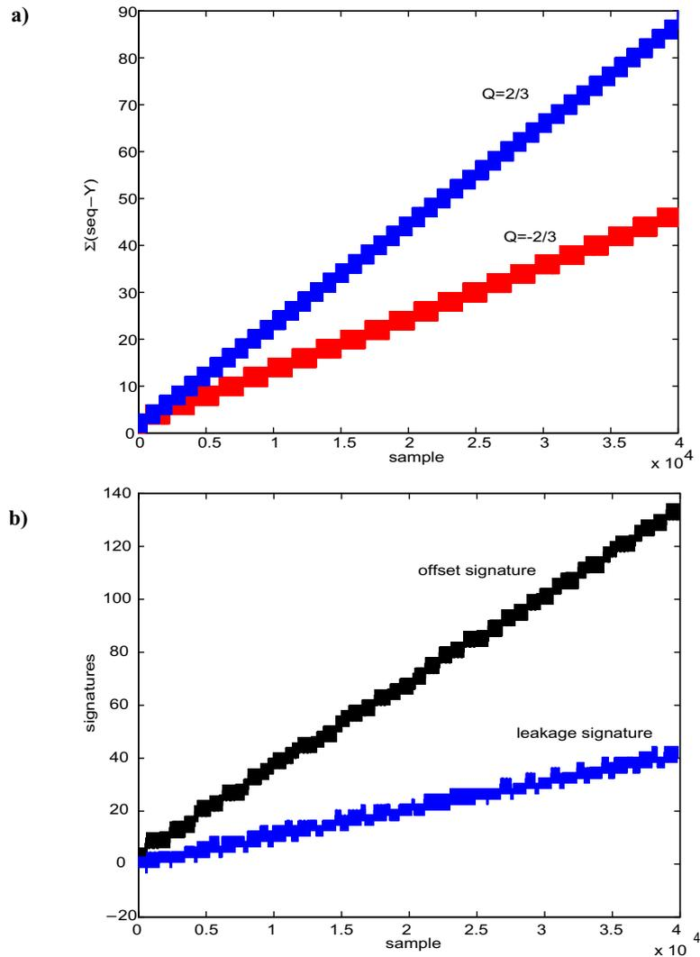
**Figure 7-23:** Evolution with time for the leakage test of the third integrator
