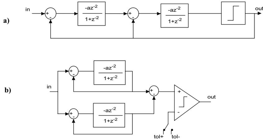
**Figure 2-11: a) double-loop bandpass  $\Sigma\Delta$  modulator; b) reconfiguration in test mode**
