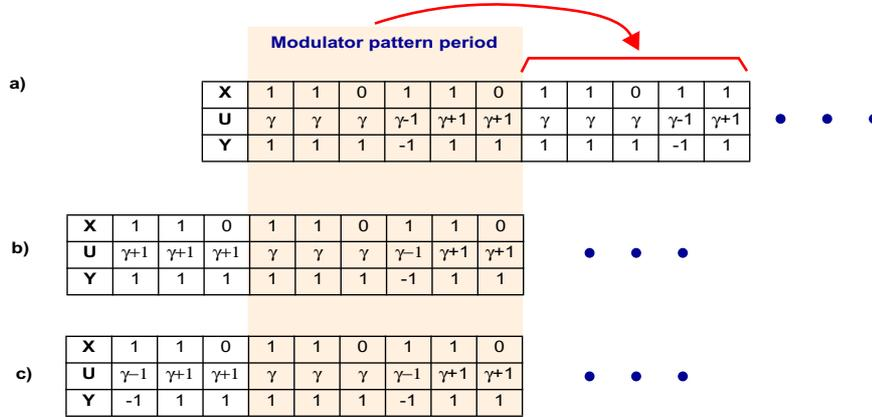
Figure 4-11: Time-domain case analysis. a) integrator initial condition  $0 < \gamma < 1$ ; b) integrator initial condition  $1 < \gamma+1 < 2$ ; c) integrator initial condition  $-1 < \gamma-1 < 0$
