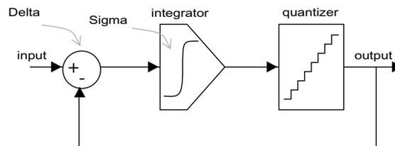
**Figure 1-3: First order  $\Sigma\Delta$  modulator diagram**
