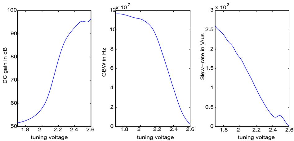
Figure 7-4: Amplifier characteristics versus tuning voltage for  $V_{tweak1}=V_{tweak2}$
