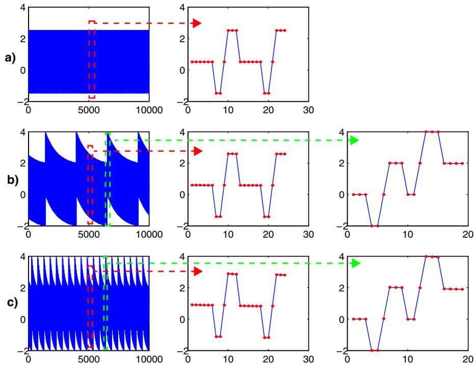
**Figure 4-25: Integrator output, for a 1st order single-bit modulator.**
