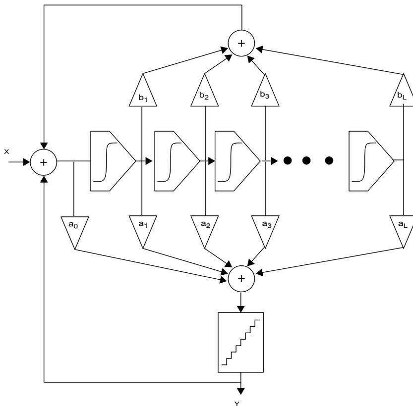
Figure 1-9: General diagram of an  $L^{\text{th}}$  order Lee-Sodini  $\Sigma\Delta$  modulator
