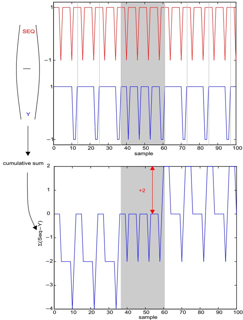
**Figure 7-25:** Leakage-induced transition in the output bit-stream and its influence on the test signature
