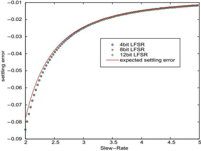
**Figure 6-5:** Modulator A settling error signature as a function of the 1st integrator Slew-rate.
