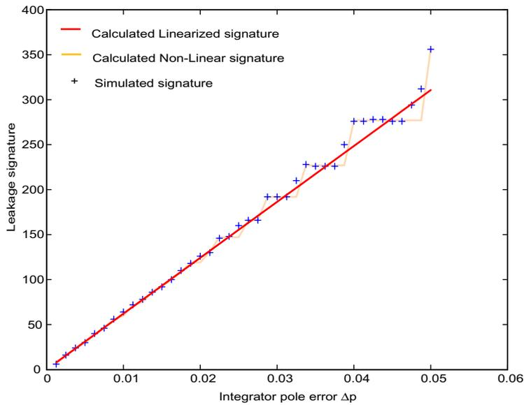
**Figure 4-34:** Test signature versus integrator leakage, for an input sequence of L=4
