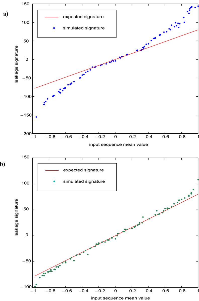
**Figure 6-8:** Modulator A (with clipping at 1.6) 1st integrator leakage signature as a function of the input sequence mean value
