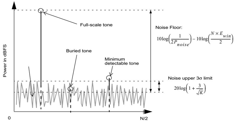
**Figure 1-25: FFT noise floor and noise dispersion**
