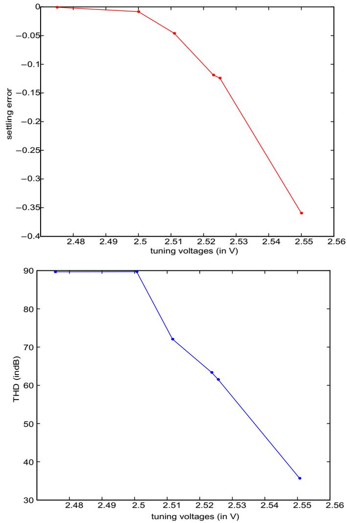
**Figure 7-36:** Correlation between the measured first integrator settling error and the measured modulator THD
