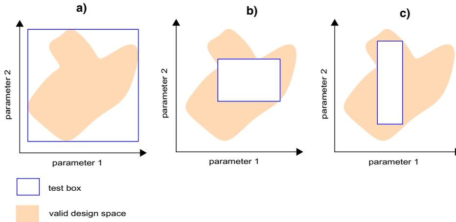
**Figure 5-23: Test box versus valid design space**
