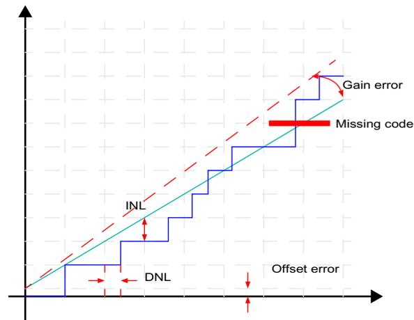
**Figure 1-18: A/D converter static metrics**
