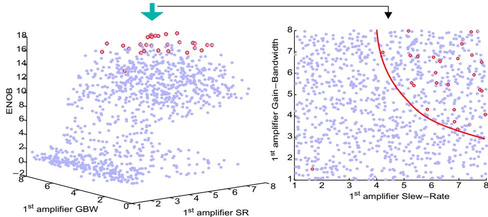
**Figure 5-22:** Cloud of points of the design space exploration representing the obtained ENOB versus the 1st amplifier Slew-Rate and Gain-Bandwidth
