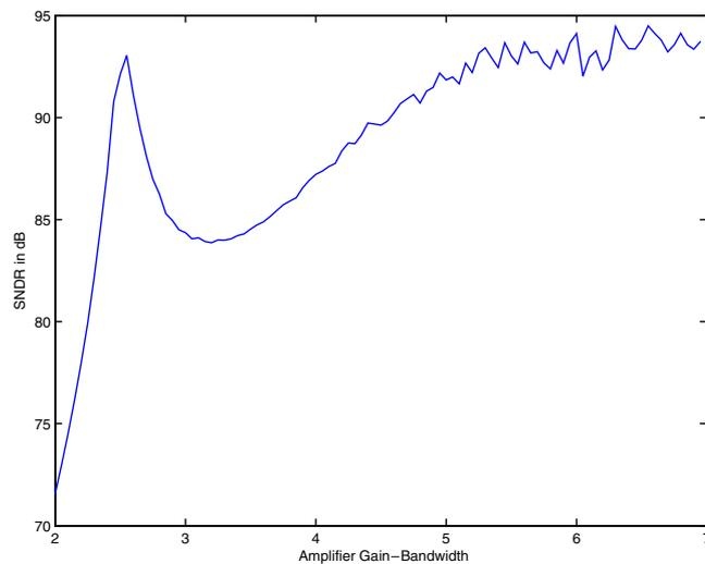
**Figure 1-17: Impact of 1<sup>st</sup> amplifier Gain-Bandwidth product on the SNDR of a 2-1 cascaded  $\Sigma\Delta$  modulator**
