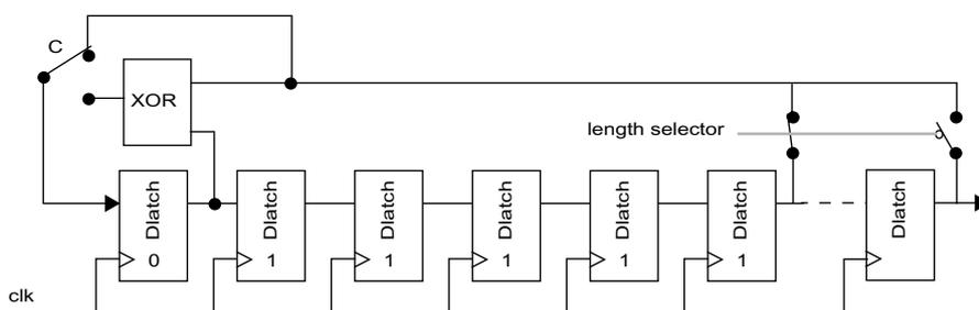
**Figure 6-9:** Test sequence generator.
