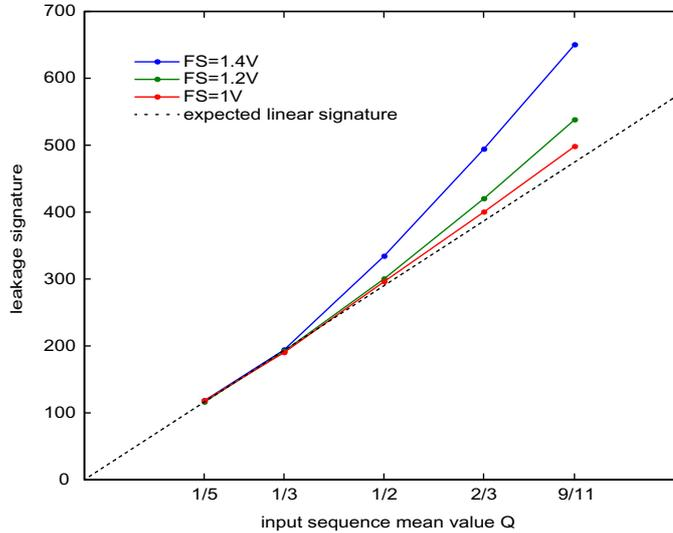
**Figure 7-32:** 1<sup>st</sup> integrator leakage signature as function of the input sequence mean value, for 3 values of the modulator Full-Scale (Vtweak2 is set to 1.8V for the 1st amplifier only)
