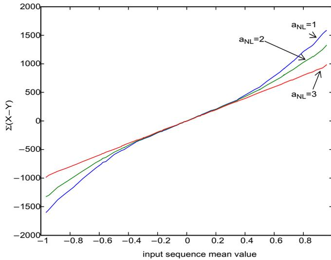
**Figure 4-38:** Sum of difference between the modulator output and the input sequence, for 3 values of the DC gain non-linear parameter  $a_{NL}$
