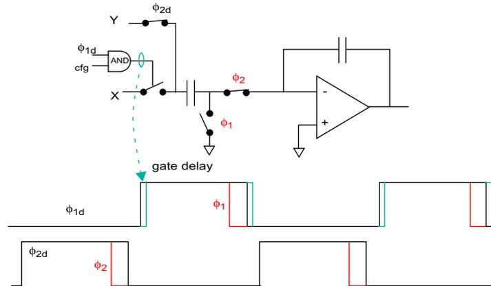
**Figure 6-18: Integrator input switch - clock gating effects**
