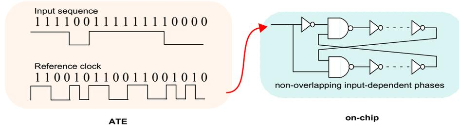
**Figure 7-9: Generation of the modulator sampling and integrating phases**
