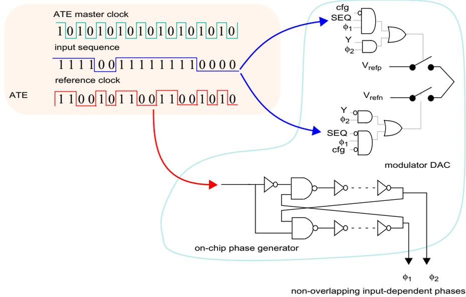
**Figure 6-29: Generation of the modulator sampling and integrating phases**
