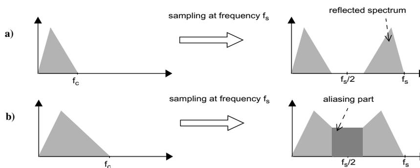
**Figure 1-2: Sampling a continuous-time signal**
