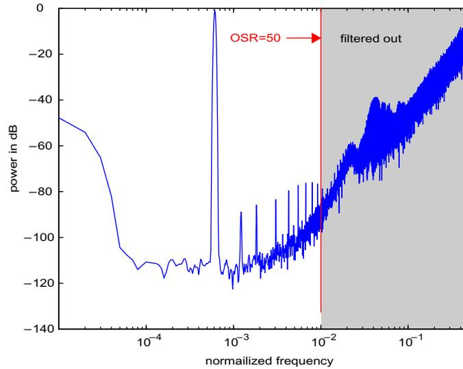
**Figure 7-21:** Nominal  $\Sigma\Delta$  output spectrum for a  $650\text{mV}_{\text{rms}}$  input sine-wave (i.e. 92% of full-scale)
