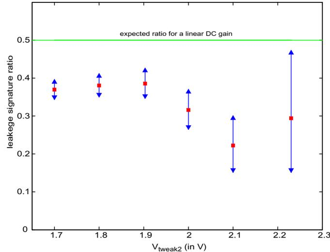
**Figure 7-31:** Measured 1<sup>st</sup> integrator DC gain non-linearity signature, as a function of the tuning voltage  $V_{\text{tweak2}}$ .
