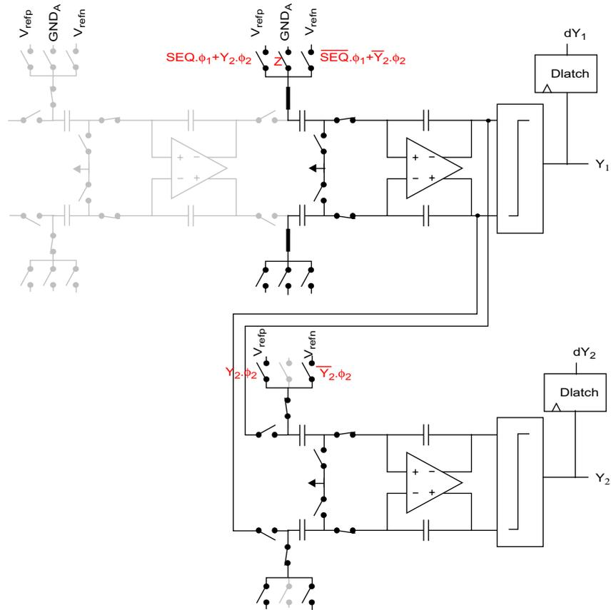
**Figure 7-14:** The  $\Sigma\Delta$  modulator reconfigured such that the 2<sup>nd</sup> and 3<sup>rd</sup> integrators form a 2<sup>nd</sup> order modulator
