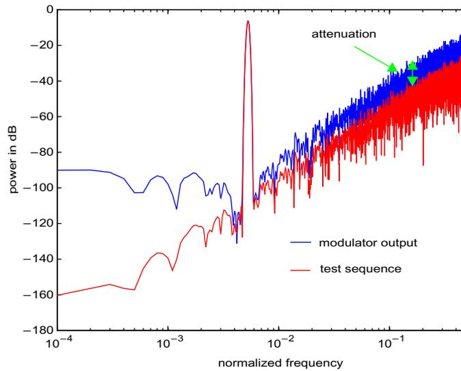
**Figure 2-12:** Input and output of the modulator under test
