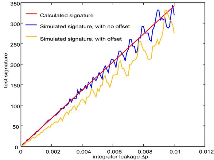
**Figure 4-31:** Second test signature versus integrator leakage, for input sequences of  $L=6$  and  $L=11$ , with and without an input-referred offset of 0.003.
