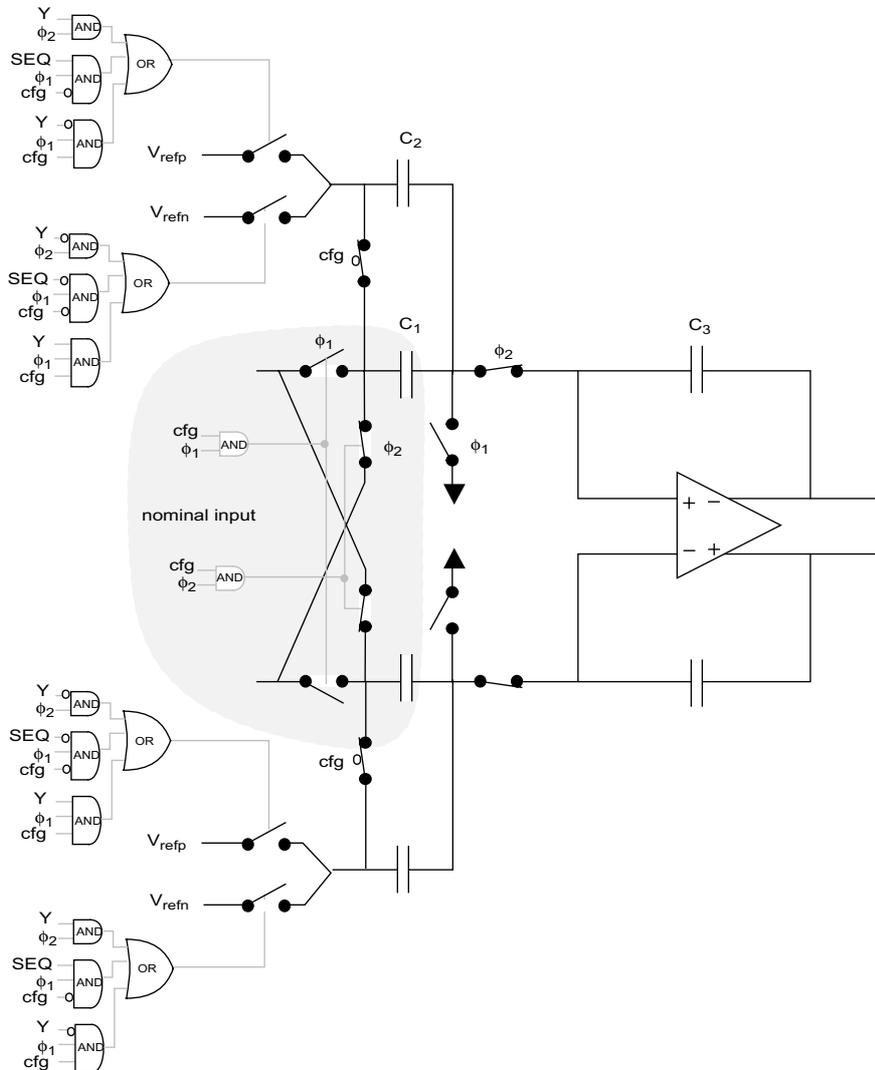
**Figure 6-25:** Disabling double sampling and connecting both input capacitors.
