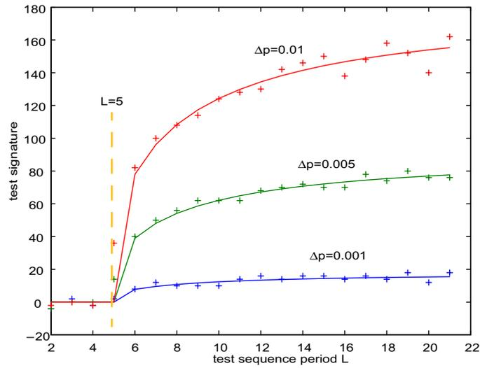
**Figure 4-26:** Test signature versus test sequence period L, for a 1st order single-bit modulator.
