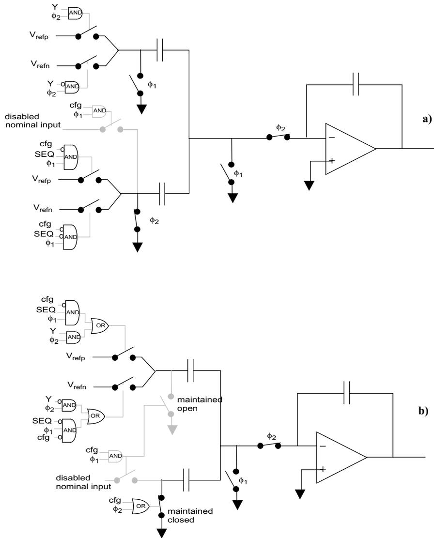
**Figure 6-22:** Digital sequence input for a double-branch integrator
