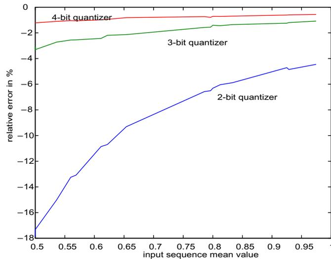
**Figure 4-24:** Relative error on the measurement of  $\Delta p$  as a function of the input sequence mean value  $Q$ .
