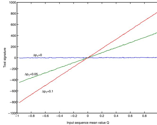
**Figure 4-14:** Test signature output as a function of the input sequence mean value
