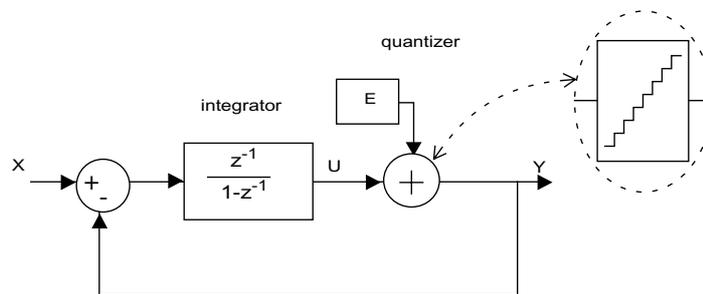
Figure 1-5: First order  $\Sigma\Delta$  modulator linearized z-domain model
