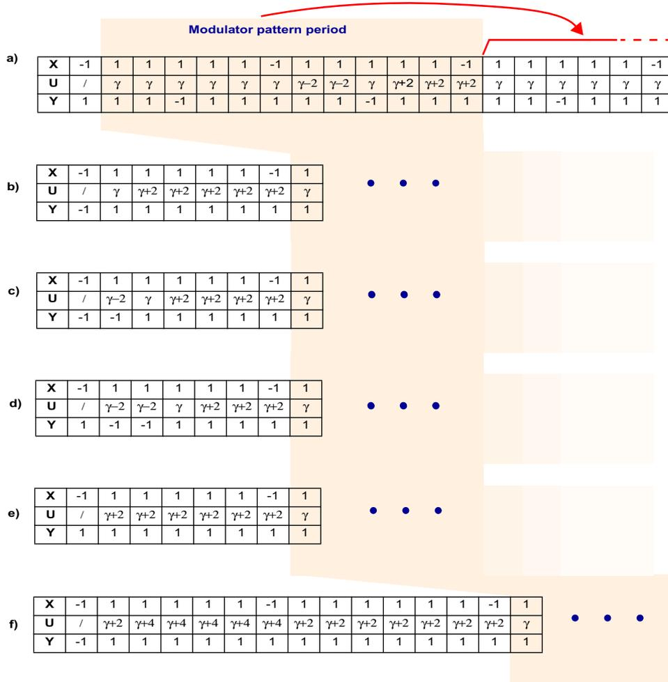
**Figure 4-8:** Time-domain case study for a [1 1 1 1 1 -1] input sequence
