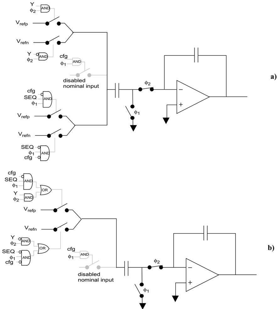
**Figure 6-21: Digital sequence input for a single-branch integrator**
