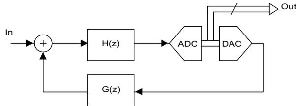
**Figure 3-4: Generic representation of a  $\Sigma\Delta$  modulator**
