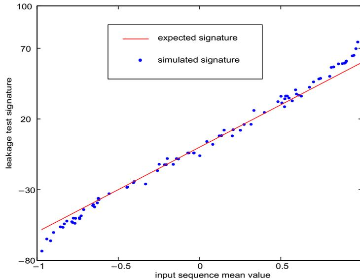
**Figure 6-4: Modulator B 1<sup>st</sup> integrator leakage signature as a function of input sequence mean value**
