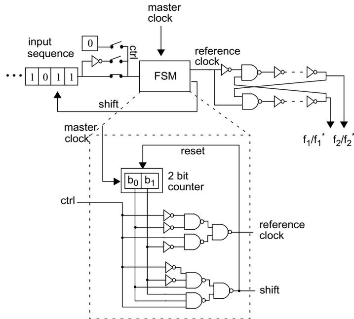
**Figure 6-30: Generation of the modulator sampling and integrating phases**
