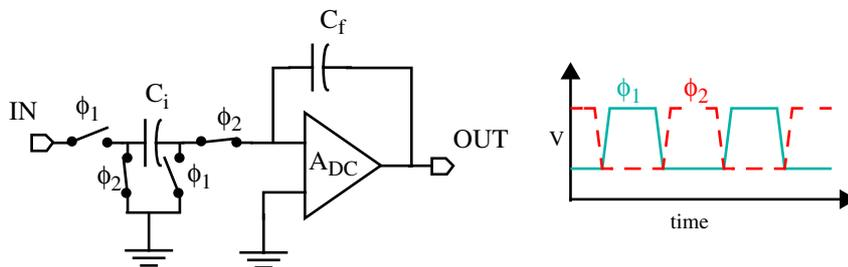
**Figure 4-1:** Switched-capacitor integrator scheme
