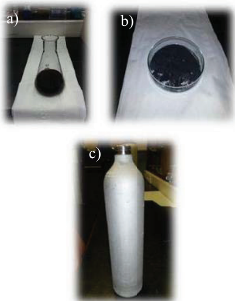
Figure 3. Products from the microwave pyrolysis: a) oil, b) solid char and c) syngas
