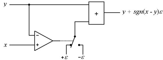
Figure 4: Circuitry implementation of CA algorithm.
