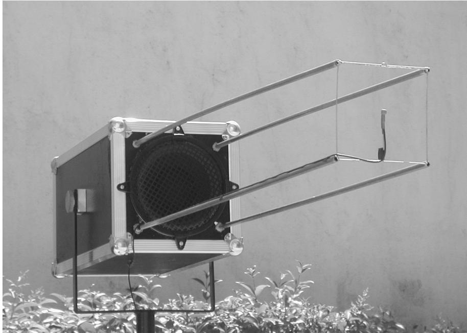
Figure 1 – The loudspeaker-microphone system
