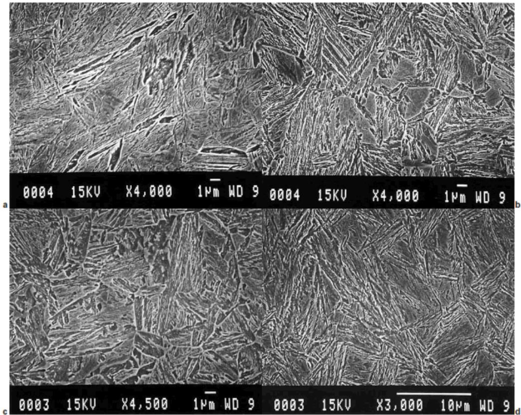
*a* Mn alloy as received microstructure; *b* Ni1 alloy as received microstructure;
