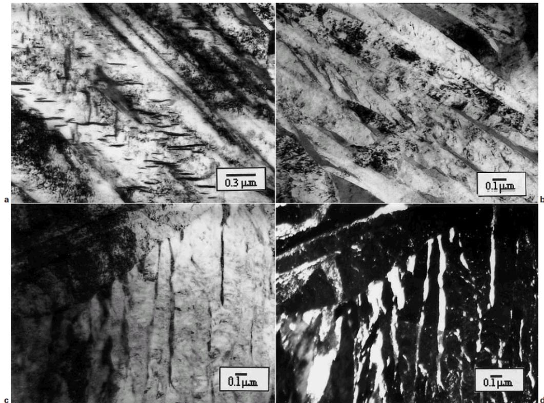
*a* Discrete carbide particles precipitate inside a martensite plate in Mn alloy; *b* None sings of recovery occur in the bainitic microstructure of Ni1 alloy; *c* Bright field and *d* dark field images reveal that retained austenite is still intact in Ni2 alloy
