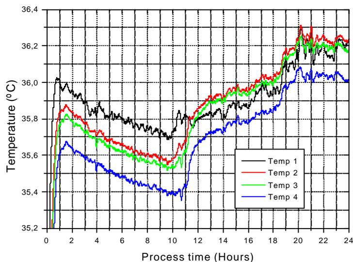
Figure 4. Temperature measurement during rennet coagulation of milk.
