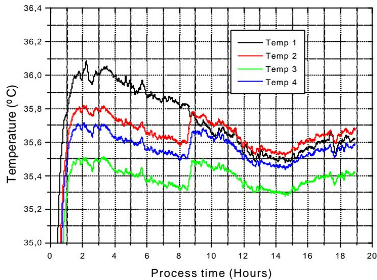
Figure 3. Temperature measurement during yoghurt milk coagulation
