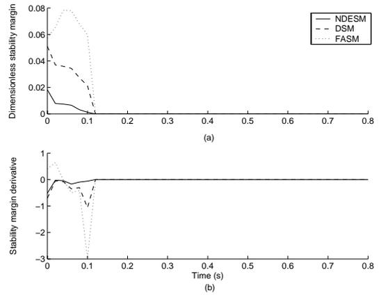
Figure 6: Unstable situation due to an external force of  $-25$  N. (a) Dimensionless DSM, NDESM and FASM; (b) Dimensionless DSM, NDESM and FASM derivatives
