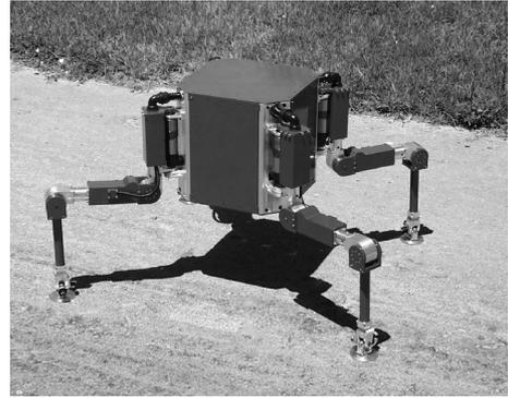
Figure 2: The SILO4 walking robot
