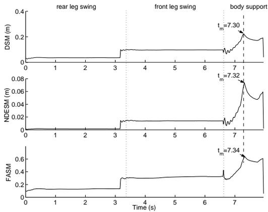
Figure 3: DSM, NDES and FASM during half a gait cycle when inertial and elastic effects arise on terrain inclined  $10^\circ$  from the horizontal plane.
