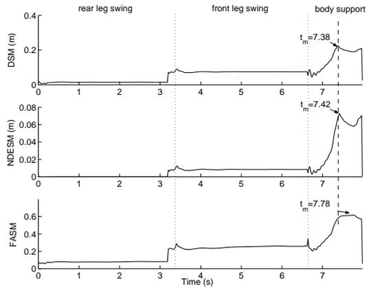
Figure 4: DSM, NDES and FASM during half a gait cycle when inertial and elastic effects arise and a 20-N manipulation force opposes robot motion on terrain inclined  $10^\circ$  from the horizontal plane.
