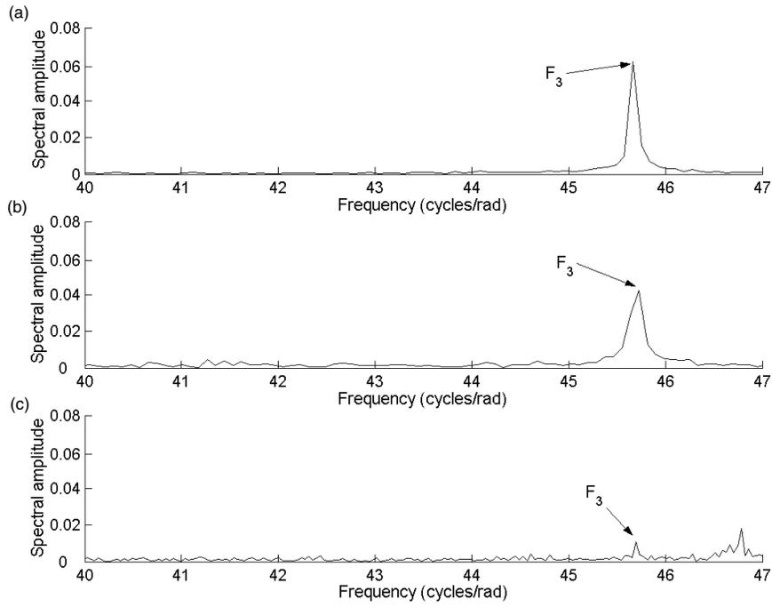
Fig. 6. Spectral component at  $F_3=45.6$  cycles/rad when the motor rotates at (a) 2000 rpm, (b) 4500 rpm, and (c) 6500 rpm.
