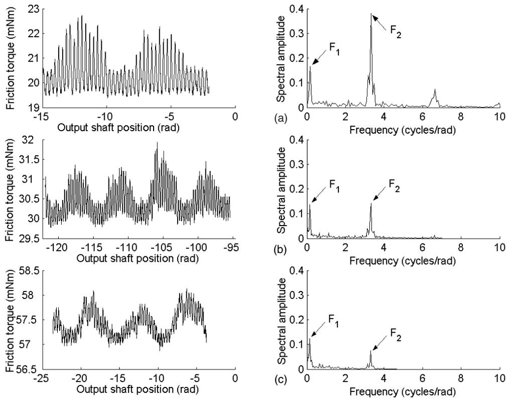
Fig. 5. Friction torque versus joint position and spectral analysis when the motor rotates at (a) 2000 rpm, (b) 4500 rpm, and (c) 6500 rpm.
