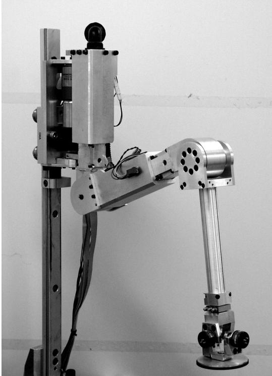
Fig. 1. Leg prototype used for friction identification.
