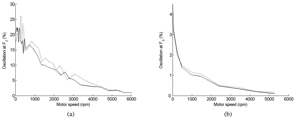
Fig. 7. Percentage of torque oscillations when rotating forwards (solid line) and backwards (dotted line) at (a)  $F_2$  and (b)  $F_3$ .
