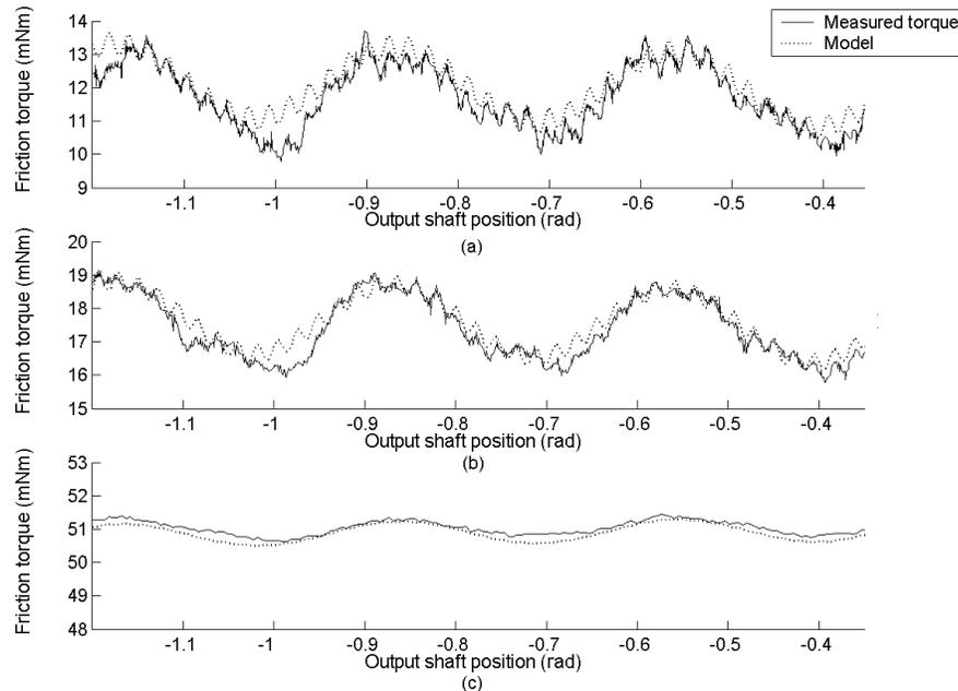
Fig. 9. Friction model validation. Comparison between real friction data (solid line) and model simulation (dotted line) for different motor speeds: (a) 280 rpm; (b) 560 rpm; (c) 3000 rpm.
