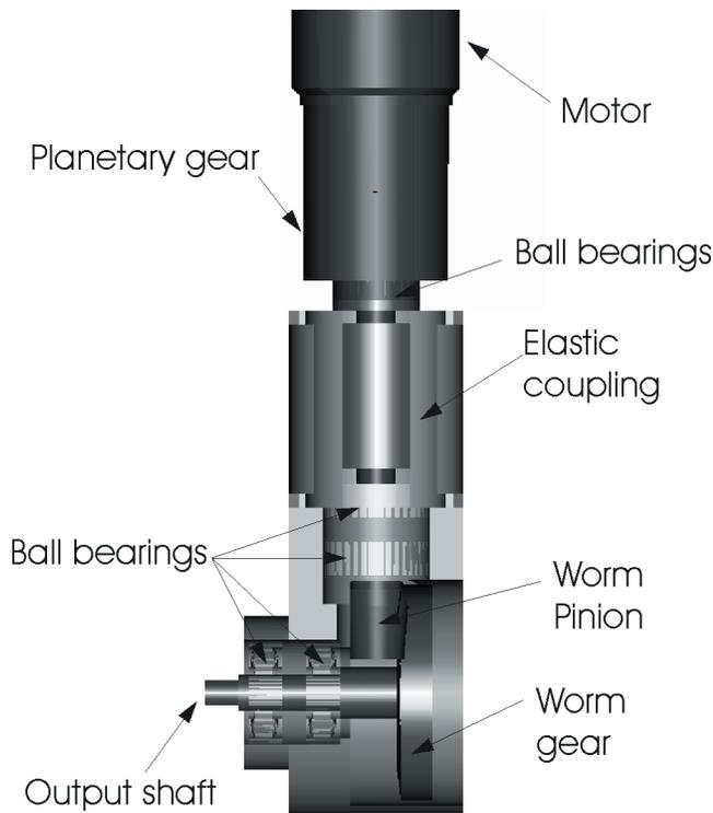
Fig. 2. Sectioned model of the joint drive and transmission system configuration.
