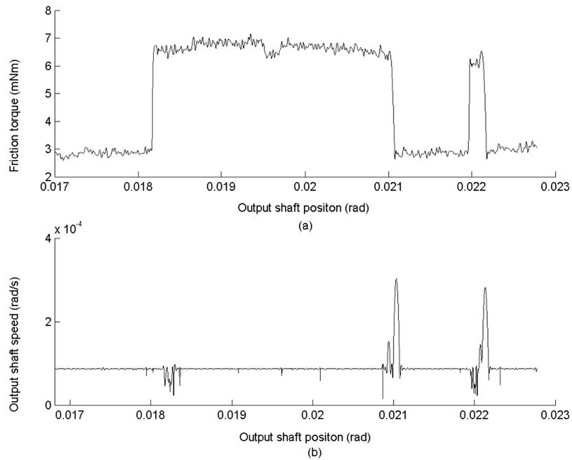
Fig. 3. Stick-slip effect at low joint velocity.
