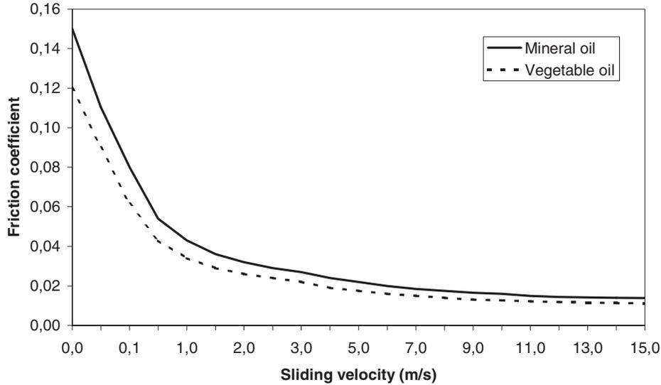
Fig. 8. Values of friction coefficient versus sliding velocity of worm gears with mineral oil-based lubricant and vegetable oil-based lubricant.
