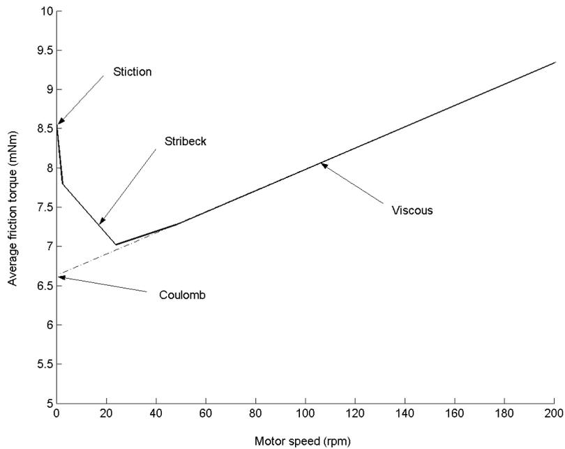
Fig. 4. Curve of average friction torque versus motor velocity, which reflects the friction components at low speeds.
