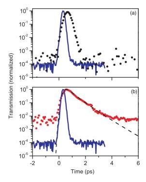
FIG. 6. (Color online) Plot of the time-resolved diffuse transmission through photonic crystals composed by PMMA spheres with n = 1.42 and a diameter d = 630 nm with  $\rho_v = 0\%$  at the passband,  $a/\lambda_1 = 0.56$  black dotted curve (a), and at the band edge,  $a/\lambda_2 = 0.59$ (b) red dotted curve. The blue solid curve is the time-resolved transmission of the pulse reference. The black dashed line represents the fit of the experimental measurement with the diffusion equation.
