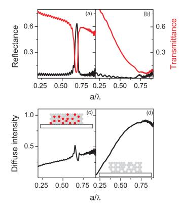
FIG. 3. (Color online) (a) and (b) The reflectance and transmittance spectra measured from samples with 0% and 40% vacancy density, respectively. Diffuse light intensity from the corresponding samples (c) before and (d) after PS removal. Notice the presence (disappearance) of the gap before (after) PS spheres removal. The insets in (c) and (d) show a schematical drawing of the corresponding samples.
