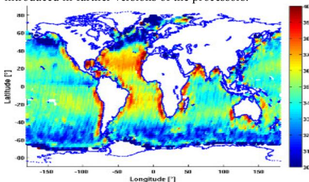
Fig. 2. Weekly global SSS map (27 April – 4 May 2010) generated from L2OS products with data weighted by their radiometric accuracy after discarding flagged values (by R. Sabia)
