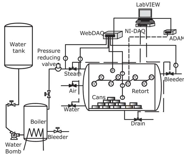
Figure 1: Schematic of a batch sterilization steam retort
