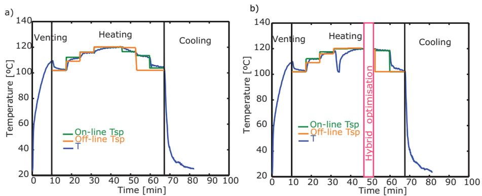
Figure 4: RTO temperature profile a) under usual perturbations and b) under a pressure drop in the pilot plant. The orange and green lines represent the off-line and on-line temperature set points.
