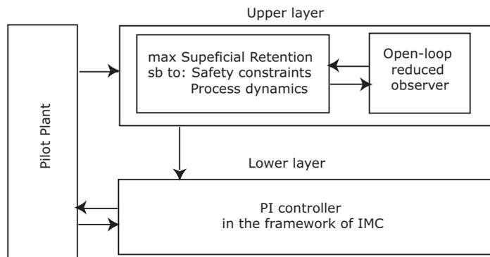
Figure 3: Real Time optimisation structure.
