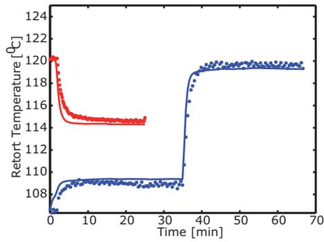
Figure 2: Validation of the model: Crosses and lines represent experimental data and the model predictions, respectively
