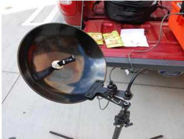
Figure 2: Parabolic wok antenna extended the range of wireless USB from 20 m to over 50 m.
