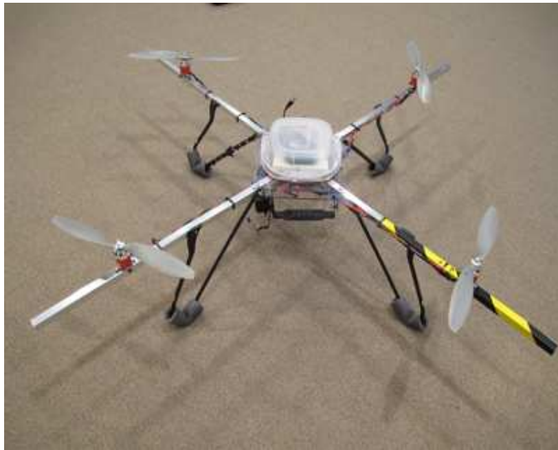
Figure 7: Four rotor multicopter. Camera tilt and pan cradle below suspended on elastic straps.
