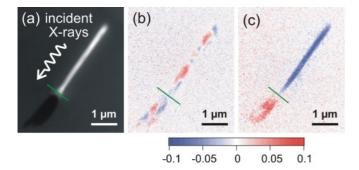
FIG. 4. (Color) (a) PEEM image of the core-shell wire taken at an angle of 0° between wire axis and incident x rays. (b) Differential XMCD image recorded at the iron  $L_3$  edge in zero magnetic field after annealing (as-prepared) and (c) after the first field sweep 120 mT  $\rightarrow$ -120 mT  $\rightarrow$  0 mT. The blue and red XMCD contrasts represent magnetizations along and antiparallel to the wire axis, respectively. The green lines mark the wire end.
