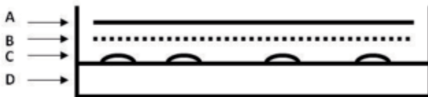
Figure 1 - Diagram of the transfer set up for the detection of mannoproteins released from yeast colonies. A, nitrocellulose membrane disc; B, sterilization filter disc; C, yeast colonies; D, agar medium in Petri dish.
