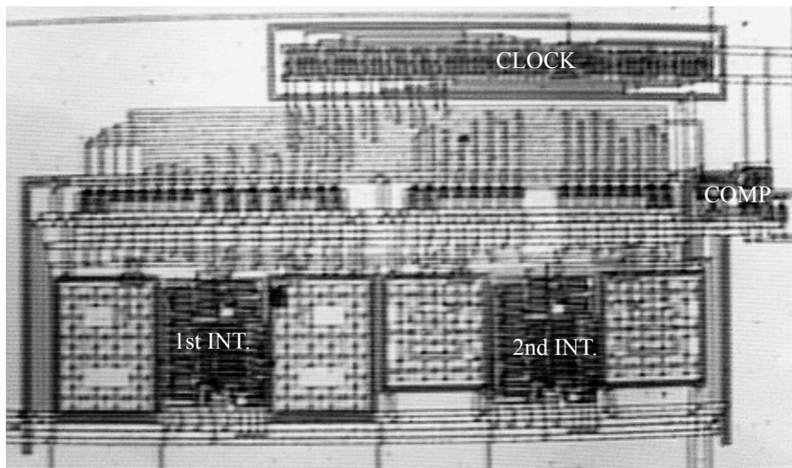
Fig. 11. Microphotograph of the second-order  $\Sigma\Delta$  modulator. Clock phase generator is also shown.
