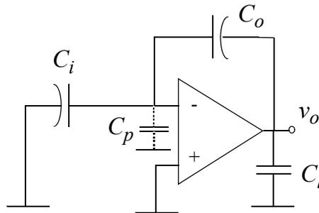
Fig. 2. SC integrator during the integration phase
