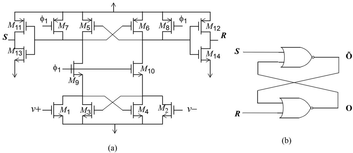
Fig. 9. Comparator. (a) Regenerative latch. (b) SR flip-flop
