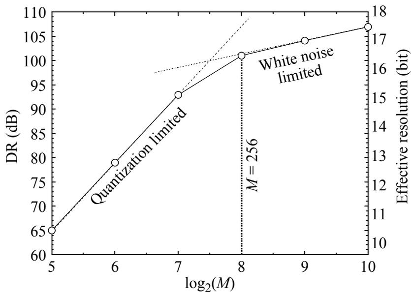
Fig. 14. Measured dynamic range versus oversampling ratio.
