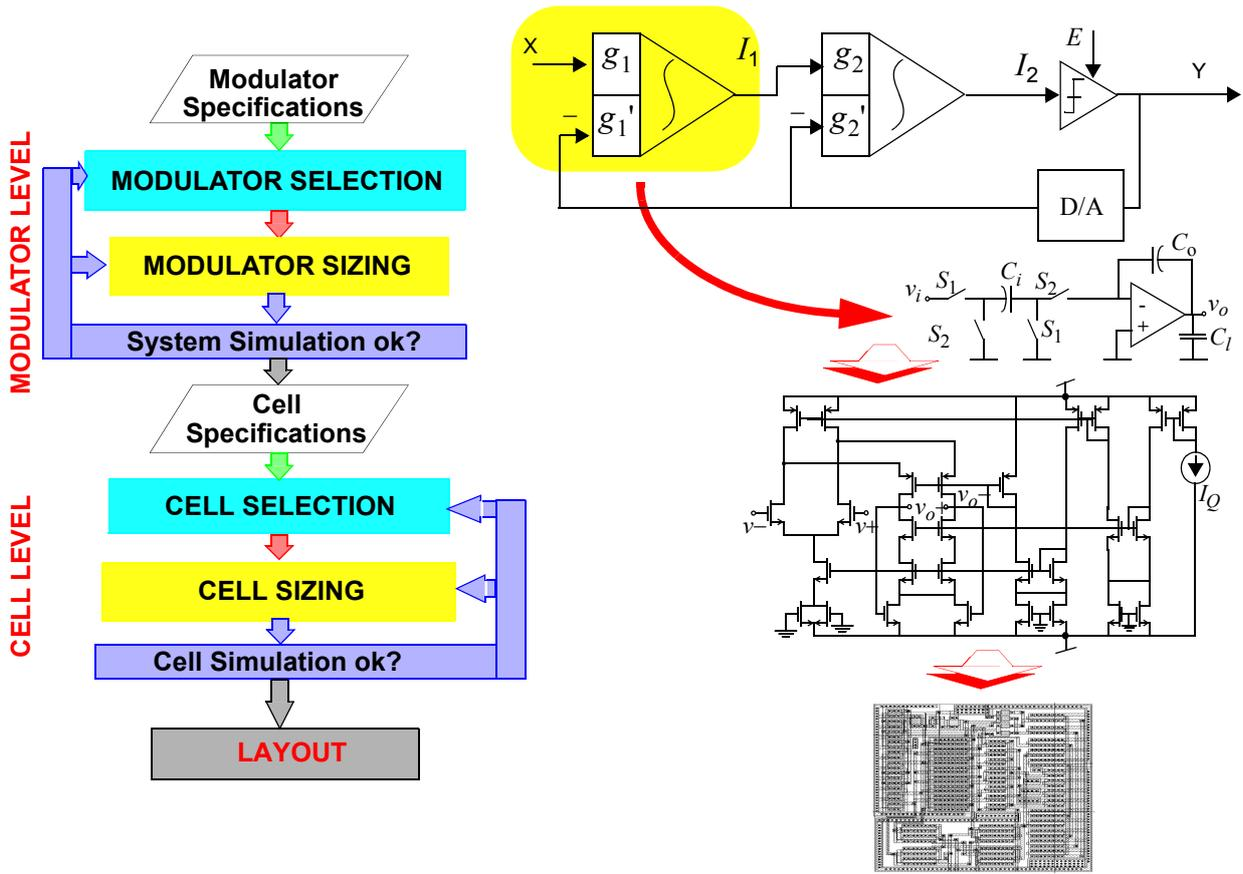
Fig. 1. Operation flow in  $\Sigma\Delta$  modulator design.
