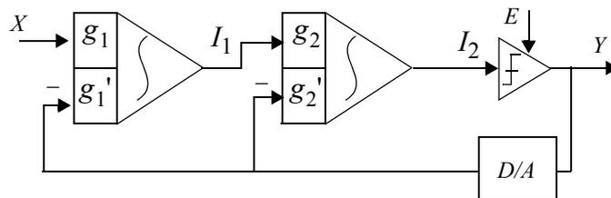
Fig. 4. Block diagram of the second-order modulator
