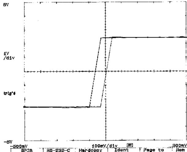
Fig. 10. Measured transfer curve of the latched comparator
