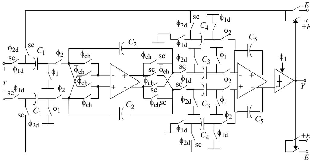
Fig. 5. Chopper-compensated SC fully-differential 2nd-order  $\Sigma\Delta$  modulator
