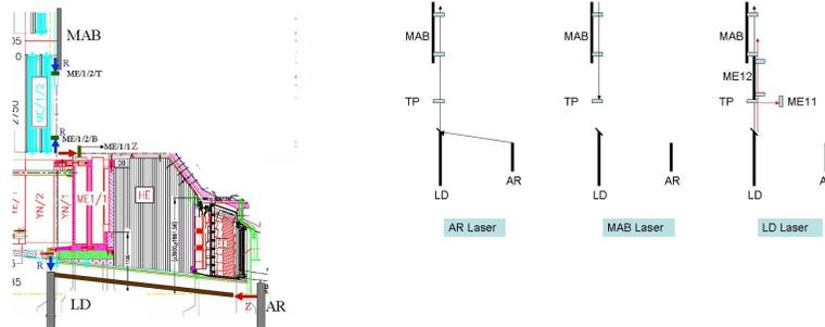
Fig. 1. Sketch of the position of the analogical proximity sensors of the Link System (left) and of the three laser paths of the Link System (right).
