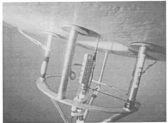
Fig. 1. underwater view of the CT recorder in buoy 1 to sample near-surface salinity
