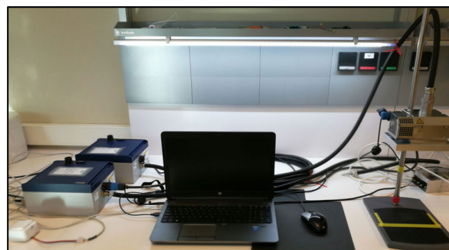
Figure 1. NIR spectrometer covering the range 1100–2100 nm.
