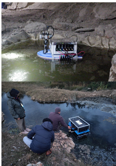
Figure 5. (top) Testing the pilot prototype of the SAM instrument during a field campaign in a natural brine pool at Boulby mine, UK, in December 2021. The campaign involved basic floatability testing of the platform material with some initial measurements of the brine for a week. (bottom) Testing the current prototype of the SAM instrument during a field campaign in a sulfidic lake at Mangalia, Romania, in October 2022. The campaign involved full floatability and maneuverability testing of the platform for an hour.
