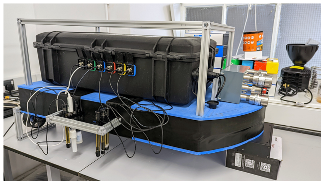
Figure 1. SAM instrument fitted with the floating platform and sub-liquid sensors (in the front of the image) and gas sensors (on the right-hand side of the image).
