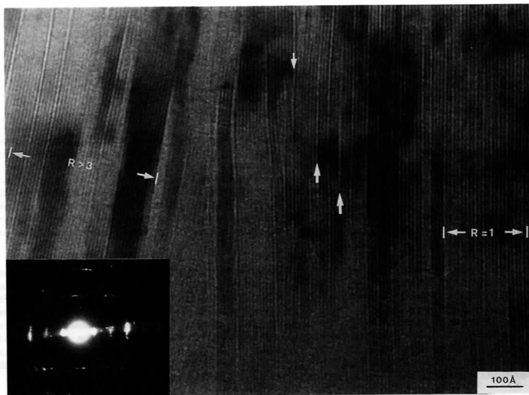
Fig. 1- HRTEM image showing coexisting R1 and R > 3 mixed layer I/S. Large arrows: separation of smectite layers due to beam-specimen interaction. Small arrow: Edge dislocation. Inset: 001 diffraction pattern of mixed-layered I/S, with weak chlorite and calcite reflections.
