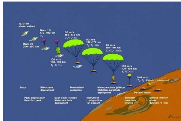
Figure 15: Entry, descent and soft landing of the European Huygens Probe. See text for details.
