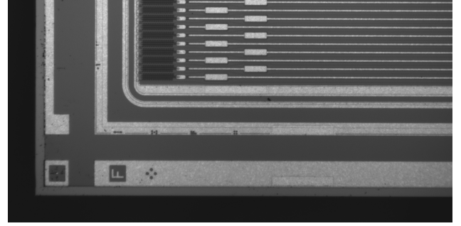
Fig. 1: Picture of the corner of an Outer Cut ATLAS12 sensor, illustrating the layout of the bias rail, guard ring, strip top metal and bias resistors. The dicing streets intended for the Inner Cut sensors are clearly visible.
