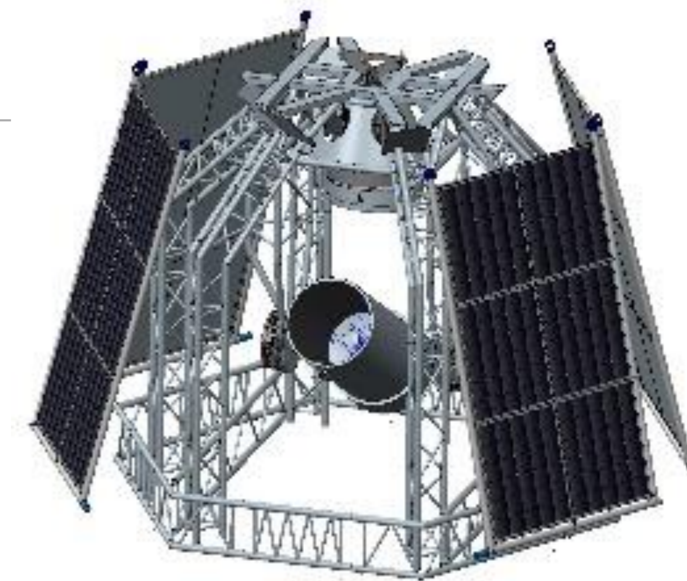
Figure 3 : CAD of the Gondola Structure [4]
