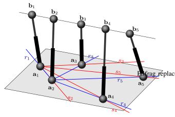
Fig. 3. A line-plane subassembly is architecturally singular if, and only if,  $CR(\mathbf{b}_2,\mathbf{b}_3,\mathbf{b}_4,\mathbf{b}_5)=CR_l(s_2,s_3,s_4,s_5)$  and  $CR(\mathbf{b}_1,\mathbf{b}_3,\mathbf{b}_4,\mathbf{b}_5)=CR_l(r_1,r_3,r_4,r_5)$ . By permuting indices, up to ten equivalent sets of conditions can be derived.
