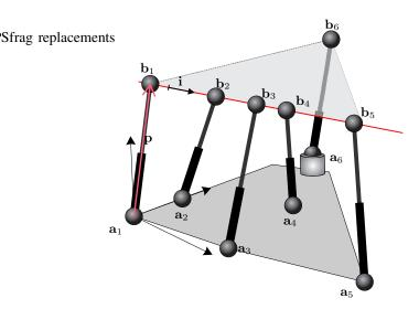
Fig. 2. Stewart platform containing a line-plane subassembly.
