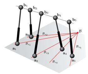
Fig. 4. The one-to-one correspondence between the attachments in the line and the lines of the pencil centered at  $\mathcal{B}$ . Each value of  $z_i$  defines a point in the line,  $\mathbf{b}_i = \mathbf{p} + z_i \mathbf{i}$ , and a line in the plane  $\mathcal{B}_{z_i}$ .
