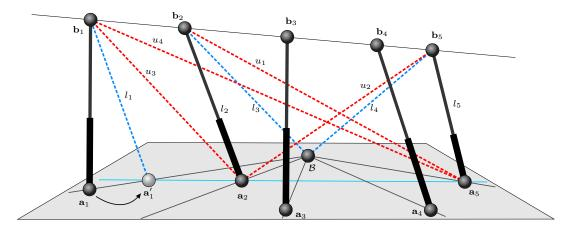
Fig. 7. The forward kinematics of a line-plane subassembly can be fully formulated in terms of distances.  $l_1$ ,  $l_3$  and  $l_4$  can be computed using the distance formula presented in Section V. Then,  $u_i$ , for  $i=1,\ldots,4$  can be obtained using standard Distance Geometry techniques.
