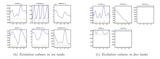
Figure 30: Volume evolution obtained in the scenario III: the minimal volume needed to satisfy the demand is, as usually, in the broken red line, while in the blue line is shown the volume evolution in the scenario III and in the broken green line the penalty volume. The last three tanks have not the minimal volume, because they are considered like a buffer.
