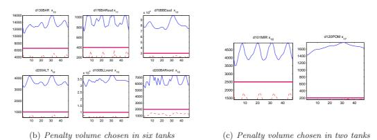
Figure 28: Penalty volume chosen considering the minimal volume showed in the Figure 27: in the broken red line it is found the minimal volume needed to satisfy the demand, in the blue line the volume evolution in the scenario I and in the magenta line the penalty volume computed.
