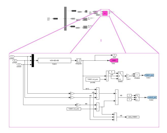
Figure 20: Tank implementation structure
