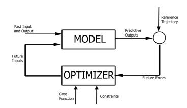
Figure 3: Basic structure of MPC
