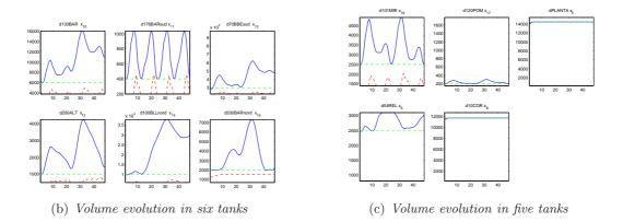
Figure 31: Volume evolution obtained in the scenario V: the minimal volume needed to satisfy the demand is, as usually, in the broken red line, while in the blue line is shown the volume trend in the scenario V and in the broken green line the penalty volume. The last three tanks have not the minimal volume, because they are considered like a buffer.
