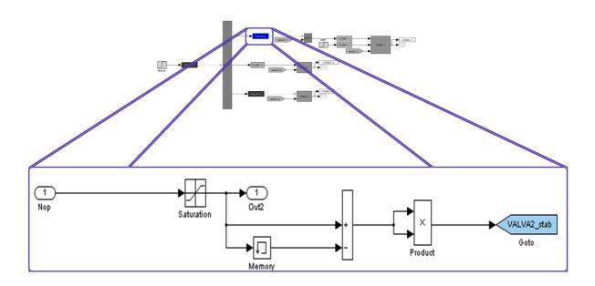
Figure 15: Implementation structure of a "normal" valve
