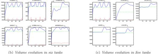
Figure 33: Volume evolution obtained in the scenario IX: the minimal volume needed to satisfy the demand is, as usually, in the broken red line, while in the blue line is shown the volume evolution in the scenario IX and in the broken green line the penalty volume. The last three tanks have not the minimal volume, because they are considered like a buffer.
