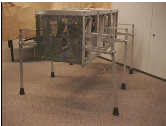
Figure 1.1: The Argos six-legged robot and its corresponding simulation.
