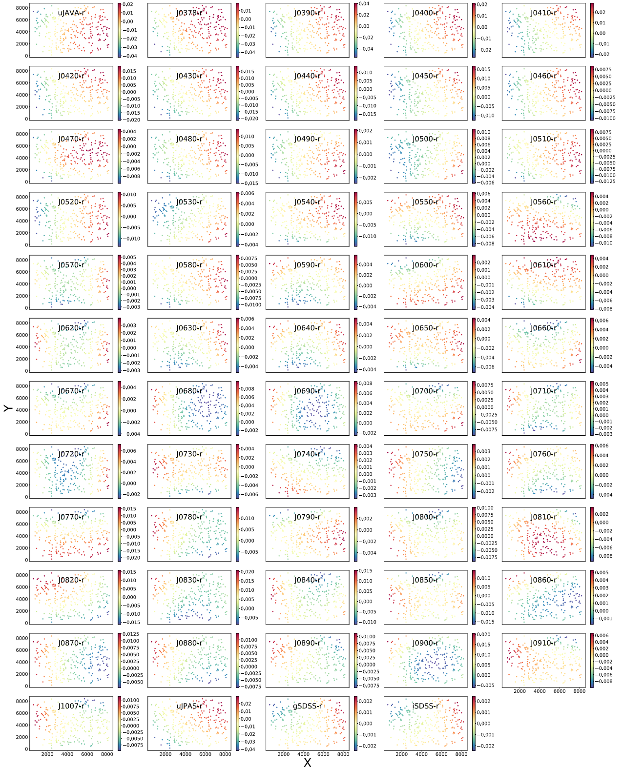
Figure 6. Flat-fielding errors in units of magnitude in the CCD focal plane for different miniJPAS colours (see text). The errors are derived by a 2D polynomial fitting as a function of CCD ( X , Y ) positions to the locus residuals. Note: the scales are different for different colours. Note: r \equiv r_{SDSS} .
