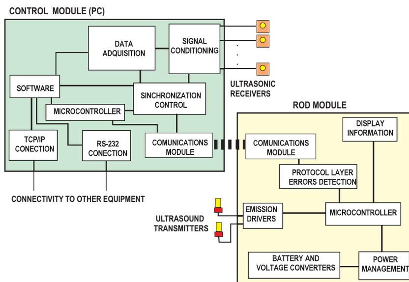
Fig. 3. General block diagram of the localisation system
