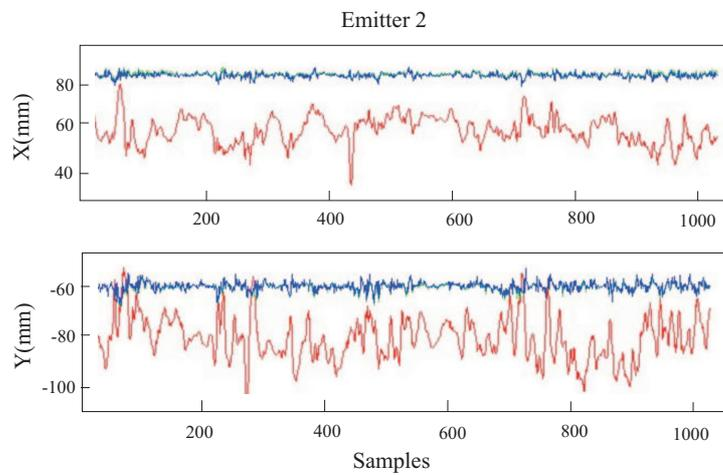
Fig. 9. (light-grey high-variance plots) X and Y estimations under a wind-flow varying between calm condition to 5 m/s speed, which suffer from errors up to 5 cm; (dark-grey low-variance plots) Same case but using the compensation method, a moderate to good compensation (1 cm error still remains) is obtained for this case where reference station is approximately 1 m apart from the real transducer position ( $x=85$  mm,  $y=-60$  mm)
