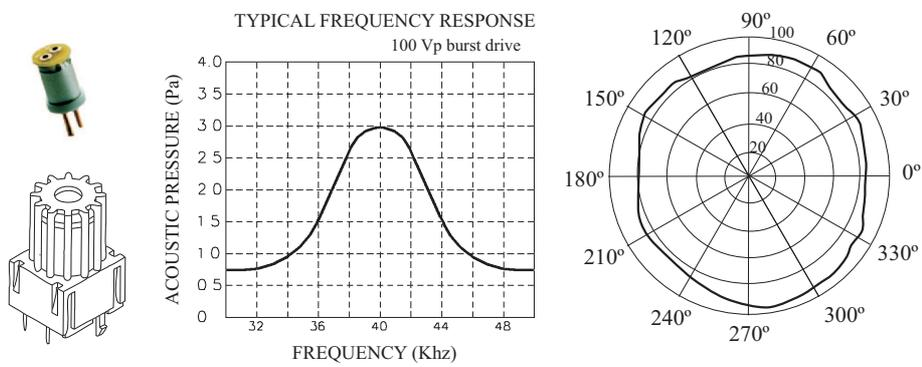
Fig. 4. Omnidirectional PVDF transducer used as emitter. (left) PVDF film is shaped in a cylindrical holding and protected with an external grid; (center) Its frequency response around 40 kHz; (right) horizontal ultrasonic emission lobe
