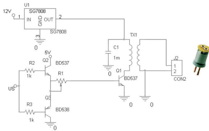
Fig. 5. Electronic circuit for ultrasonic PVDF excitation
