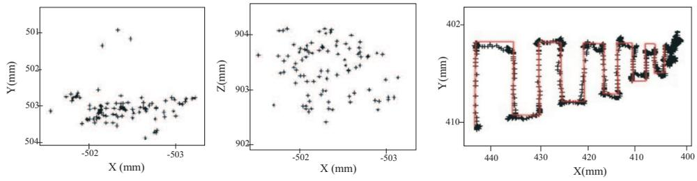
Fig. 8. (left-middle) Accuracy and repeatability indoors tests showing the dispersion in 3D position estimation; (right) Resolution indoors tests performed following a predefined increasing-size pulse-like path
