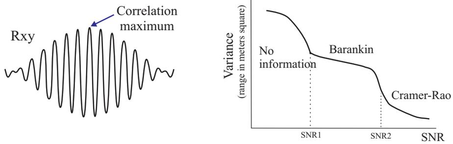
Fig. 6. (left) result of correlating the received signal with the stored reference; (right) Regions where estimation variance changes with SNR at certain thresholds. This thresholds change with bandwidth, duration and frequency of signals
