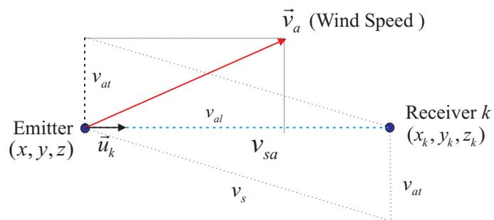
Fig. 7. Air flow components  $\vec{v}_a = \{v_{al}, v_{at}\}$  with respect to the emission-reception axis
