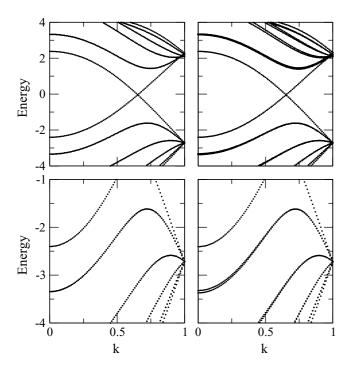
FIG. 9. Band structure of the armchair (5,5) carbon nanotube calculated with  $\lambda = 0$  (top left) and  $\lambda = 0.4$  eV (top right). Bottom panels represent a zoom of the corresponding bands between -4 and -1 eV. *k* are in units of  $\frac{\pi}{a}$ .
