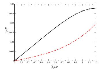
FIG. 2. (Color online) Energy splitting for the conduction (circles) and valence (diamonds) bands of the (61,0) zigzag CNT as a function of the value of the spin-orbit coupling constant  $\lambda$ . The solid (black) and dashed (red) lines are a guide to the eyes.
