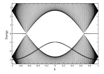
FIG. 3. Band structure of the zigzag ribbon n = 60 obtained with SOI  $\lambda = 0.4$ . *k* are in units of  $\frac{\pi}{a}$ .
