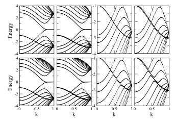
FIG. 8. Band structure of the N = 10 zigzag flat (upper part) and curved (lower part) nanoribbon. (Left to right) Calculated with  $\lambda = 0$  and  $\lambda = 0.4$  eV. The two last panels show a detail of the bands, limiting the energy axis between -4 and -1 eV (see text). *k* are in units of  $\frac{\pi}{a}$ .
