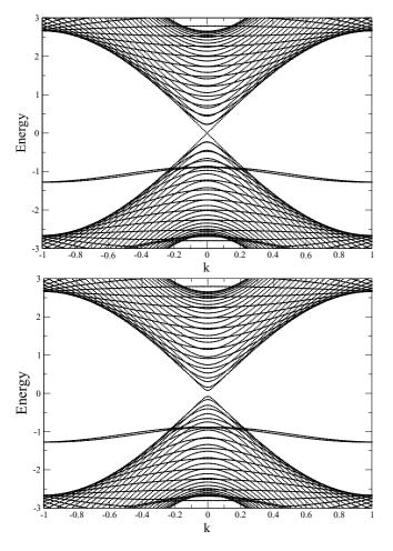
FIG. 7. Band structure of the armchair N = 62 metallic ribbon (top) and N = 60 semiconductor ribbon (bottom) with SOI  $\lambda = 0.4$ . *k* are in units of  $\frac{\pi}{a}$ .
