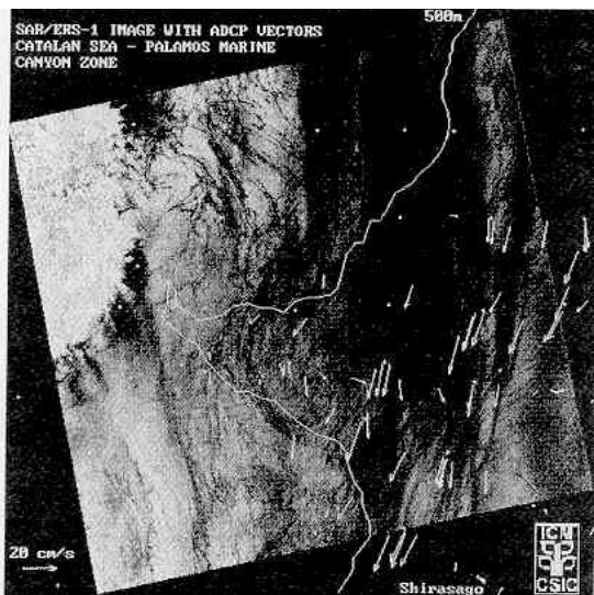
Figure 1 ERS-1 SAR subscene 50 x 50 km on 15 May 1992 superposed to surface ADCP vectors and location of the canyon (500 m isobath). Pixel size is 100 m
