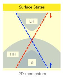
FIG. 1. Incorrect picture of surface states obtained after neglecting the coupling to the heavy-hole (HH) band. The surface states are formed in a two-band model consisting of electrons (e) and light holes (LH) in an inverted-band semiconductor.
