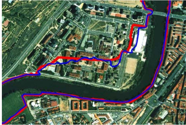
Figure 5. Ortho aerial photograph showing the flood outer limits (black line). The thicker grey line marks the limit of the 500 year flood estimated by the Confederación Hidrográfica del Duero.
