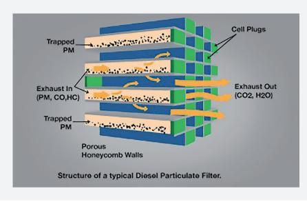
**FIGURE 3**–Honeycomb system treating gases and soot from industrial Diesel motors. Source: http://urbanemissions.blogspot.com/2015/12/what-is-diesel-particle-filter-dpf.html.
