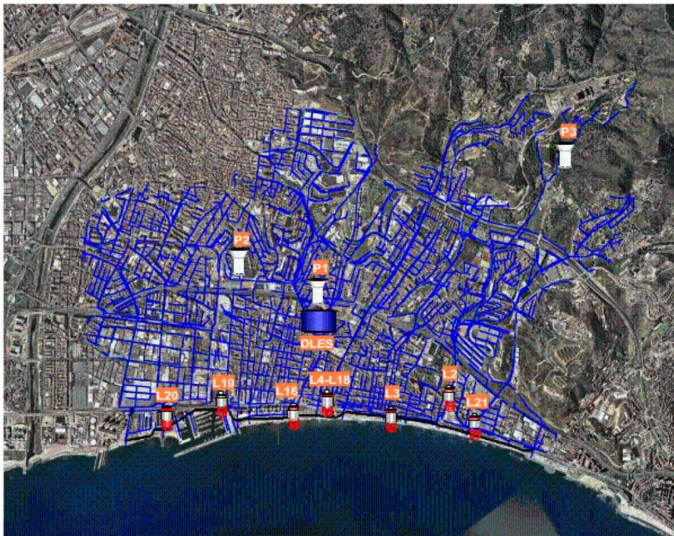
Figure 3 | Map of the Badalona SN. The tank is marked as DLES, while the LX elements are CSO points (Sun et al. 2020). Please refer to the online version of this paper to see this figure in colour: https://doi.org/10.2166/hydro.2021.149 .
