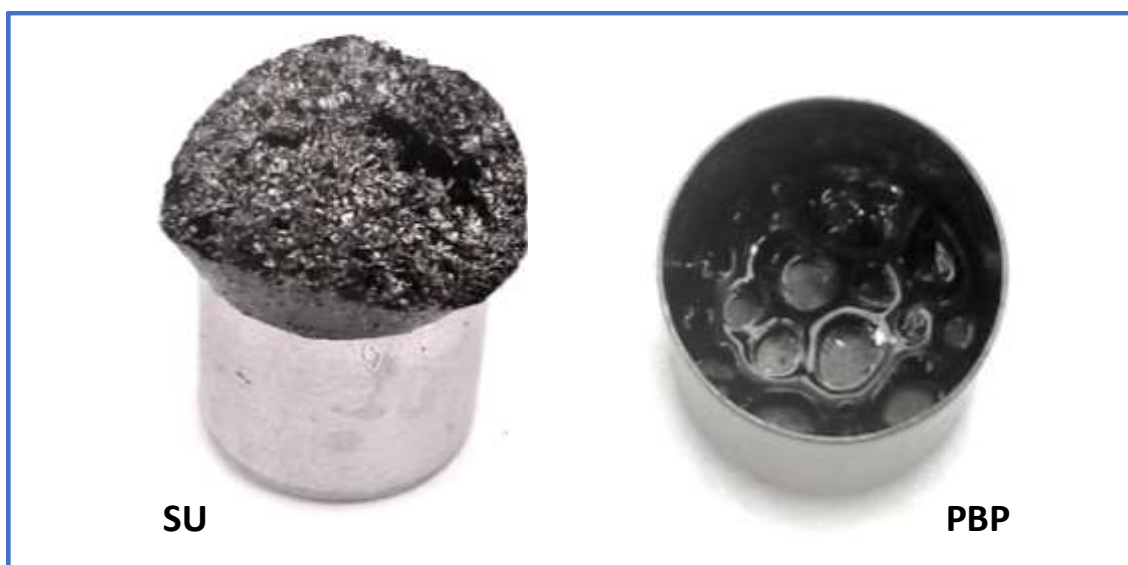
Fig. S1. Residues of the TGA experiments carried out at 500 °C with SU and PBP.
