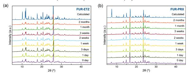
**Figure 7.** PXRD patterns of FUR–ETZ (**a**) and FUR–PRX (**b**) with respect to the stability under accelerated ageing conditions (40 °C, 75% RH) at different time intervals.
