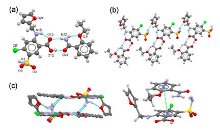
**Figure 2.** (a) Asymmetric unit of the FUR–ETZ cocrystal. (b) acid… amide and sulfonamide… furan synthons give a ribbon along the *b*-axis by H-bonding interactions (Table S1). (c) Left. Detail of the column structure in FUR–ETZ. Carbon bound H atoms omitted for clarity Right.  $\pi$ – $\pi$  stacking interaction in the FUR–ETZ cocrystal.
