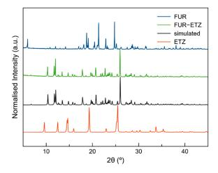
**Figure 1.** PXRD patterns of the new phase FUR–ETZ obtained by liquid-assisted grinding (LAG) with methanol (MET) solvent, the simulated pattern from crystal structure and the corresponding reactants.
