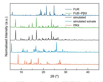
**Figure 3.** PXRD patterns of the new phase FUR–PRX obtained by liquid-assisted grinding (LAG) with methanol (MET) solvent, the simulated patterns from crystal structure and reported acetone solvate structure and the corresponding reactants.
