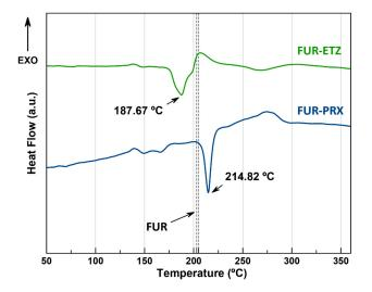
**Figure 6.** Differential scanning calorimetry (DSC) plots of FUR–ETZ and FUR–PRX. Dotted lines correspond to the range of temperature reported for melting of FUR.
