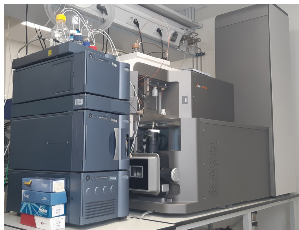
The recently installed high-resolution mass spectrometry facility in the Scientific Instrumentation Service: Shown is the UPLC (ultra-performance liquid chromatography) instrument (on the left) linked to the high-resolution electrospray ionization mass spectrometer Vion IMS-QToF (on the right)
