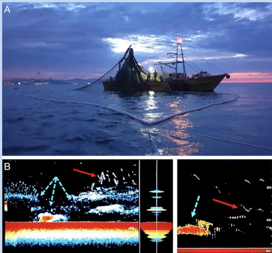
Figure I: Purse seining fishing of small pelagics. Fisheries-induced changes of shoaling behaviour can make fish hard to locate and capture for fishers with socio-economic repercussions on fisheries and local communities. A) a purse seiner fishing boat hauling in the net. B) imaging of an echo sounder on a purse seiner during small pelagic fishing in the North-Western Mediterranean Sea (light-blue dashed arrows indicate shoals of small pelagics, and red solid arrows indicate tunas). Photos copyrighted and courtesy of the Catalan Institute for Ocean Governance Research / Susana L. Díez González and Josep Palaus.
