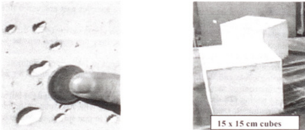
Figure 6: Surface appearance of conventional (left) and SCC (right) concretes
