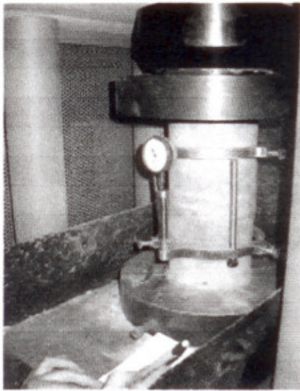
Figure 4: Static Elasticity Modulus for SCC-I and SCC-II according to ASTM C-469
