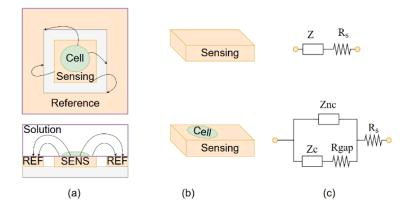
**Fig. 2.** Electrical models for cell culture over a sensing electrode. (a) TOP and SIDE views of the cell adhered to the electrode substrate immersed on an ionic solution. Two stages are depicted (and modeled); empty electrode (b) and partially covered electrode (c).
