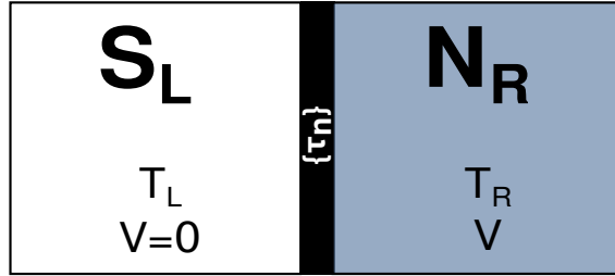
Figure 4.2: Resistive junction between a metallic and a superconducting electrodes with tuneable transmission. Both reservoirs are at the same temperature but electrostatically biased by a potential V .
