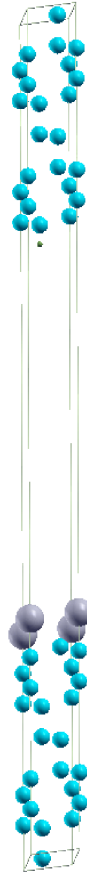
Figure A.1: Schematic representation of the Tl/Si(111) surface slab with a hydrogen overlayer covering the opposite side of the slab. Grey, blue and green balls denote Tl, Si and H atoms, respectively.
