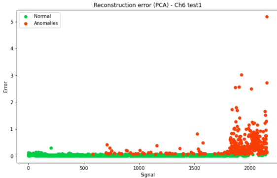
Figure 3.39: Reconstruction error and classification of anomalies (PCA - GMM), channel 6, test 1.
