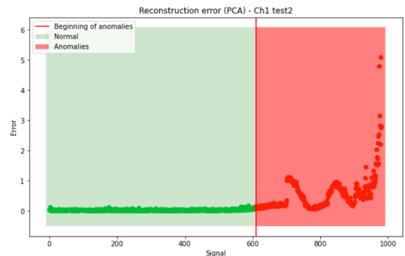
Figure 3.27: Reconstruction error and beginning of anomalies (PCA - Z-Scores), channel 1, test 2.
