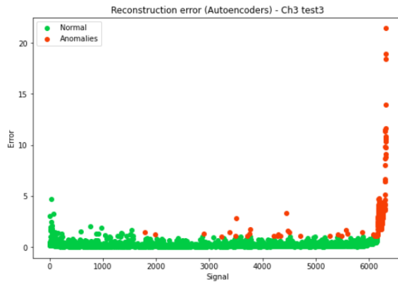
Figure 3.50: Reconstruction error and classification of anomalies (Autoencoder - Z-Scores), channel 3, test 3.
