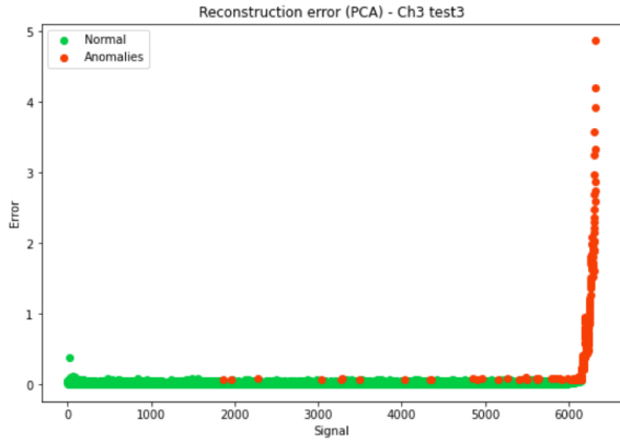
Figure 3.31: Reconstruction error and classification of anomalies (PCA - Z-Scores), channel 3, test 3.
