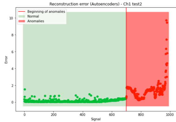
Figure 3.45: Reconstruction error and beginning of anomalies (Autoencoder - GMM), channel 1, test 2.
