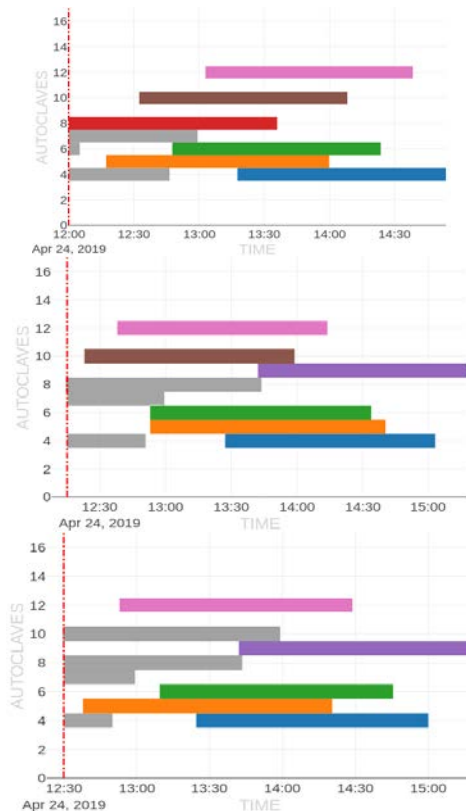
Fig.9 Three consecutive Gantt charts obtained every 15 minutes. Vertical red line represents current time.
