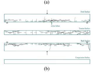
Figure 8: Crack pattern of the beam
