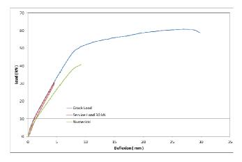
Figure 9: Curve of the deflection of the central region of the beam versus the external load (numerical and experimental data)
