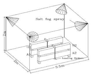
Figure 3: Environment an load condition of the bean.
