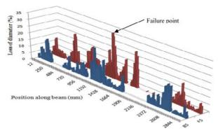
Figure 7: Loss of diameter of reinforcement along the length.
