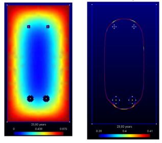
(b) (B) **Figure 5:** Chloride concentration distribution not considering the presence of the micro-craks after 24 years.
