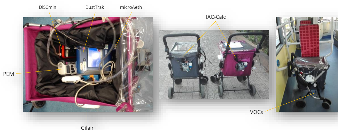
Figure 1. Equipment used during the BUSAIR campaigns measuring air pollutants inside public buses.
