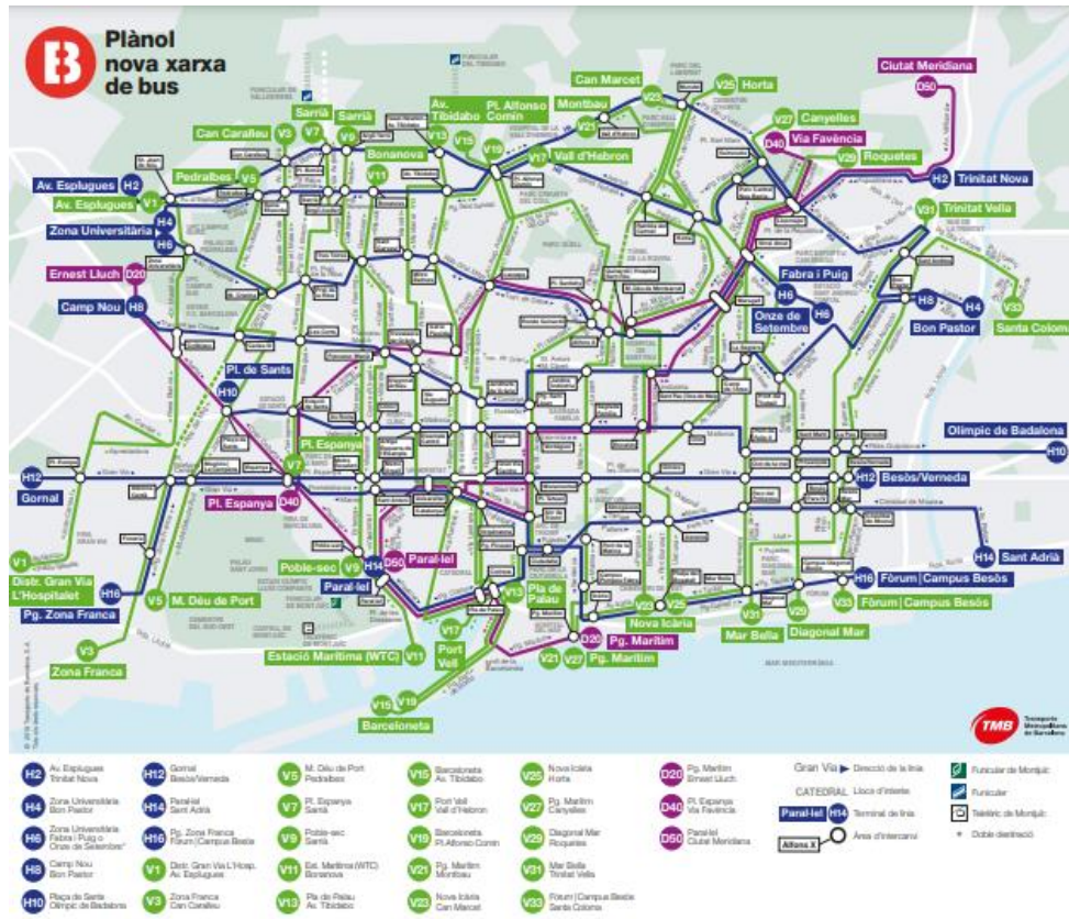
Figure 2. Bus routes in the Barcelona public transport system, separating vertical (V) and horizontal (H) routes (source: TMB)
