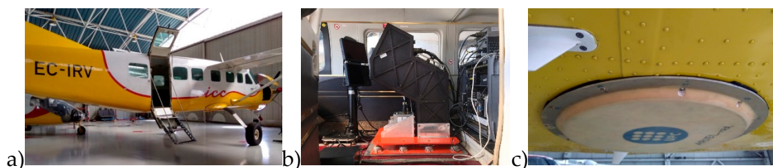
Figure 4. Experiment instrumentation: (a) CESSNA Caravan plane, (b) AISA (hyperspectral VNIR) and TASI (TIR), and (c) ARIEL L-band radiometer.
